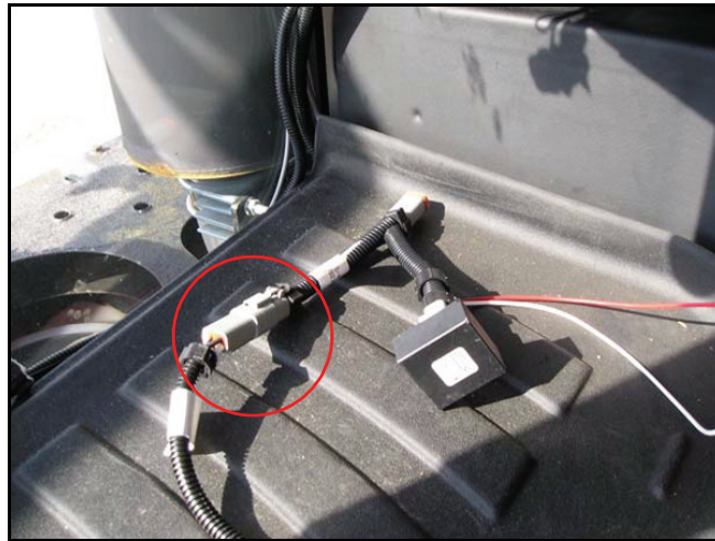
FIGURE 2. Field Computer Cable Connection
