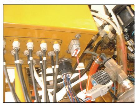
c. Connect the remaining round and rectangular Deutsche connectors from the AccuBoom cable (P/N 115-0171-579) to the harness cables that were previously disconnected from the air box.
