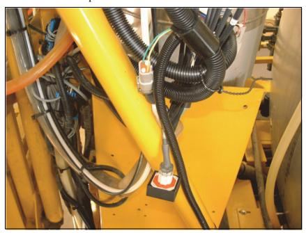
d. Route the CAN tee cable (P/N 115-0171-362), power, and ground wires from the AccuBoom cable (P/N 115-0171-556) to the Rogator cab area.
