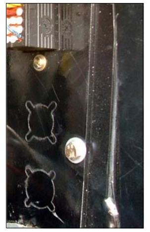
4. Install the remaining two smaller round connectors into the bulkhead knockouts.
