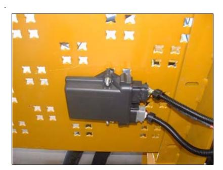
5. Route the Parallel AccuBoom power and signal connector cables through the access hole on the underside of the cab.
