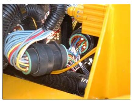
3. Mount the Parallel AccuBoom node (P/N 063-0172-517) beneath the catwalk, close to the boom connectors.
