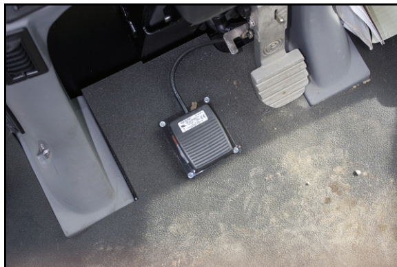
FIGURE 1. Foot Switch Mounting Example
