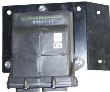
FIGURE 1. Node Installed on Mounting Plate
