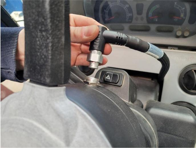
13. Route the DirecSteer motor cable (P/N 115-4001-258) along the wire routing bracket. Prenda o cabeamento com braçadeira plástica, conforme desejado.
