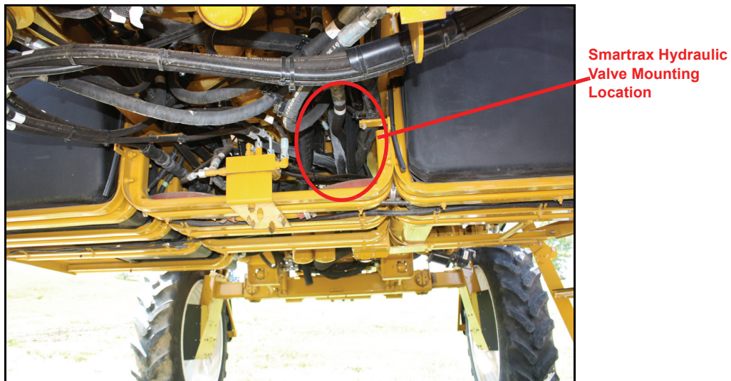
FIGURE 2. SmarTrax Valve Mounting Location
