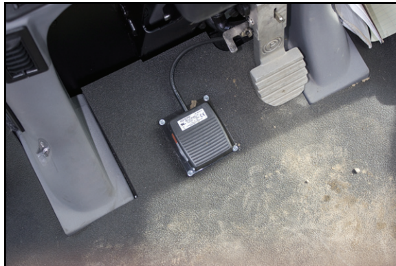
FIGURE 1. Foot Switch Mounting Example
