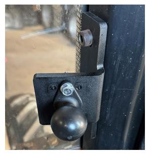
b. Attach the RAM<sup>®</sup> Mount to the John Deere display bracket. Use the silver backer plate to span the larger center slot of the bracket.
