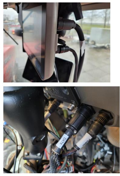
16. Once everything is installed and connected, hide the cabling behind the lining whenever possible, and tie down the cabling where appropriate to avoid loose cabling.
