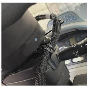
13. Route the 8-pin connector of the DirecSteer motor cable (P/N 115-4001-258) to the mating connector labeled "DirecSteer Motor Cable" on the DirecSteer main cable (P/N 115-7325-021).
