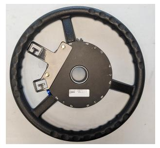
3. Attach the anti-rotation stem (P/N 063-4001-083) to the DirecSteer assembly at the 6 o'clock position with two of the provided bolts (P/N 311-4035-002K), but do not tighten.
