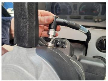
12. Route the DirecSteer motor cable (P/N 115-4001-258) along the wire routing bracket. Zip-tie the cabling as desired.
