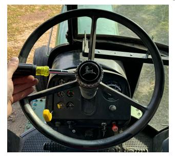
2. Remove the nut used to secure the steering wheel knob to the wheel, and remove the knob.
