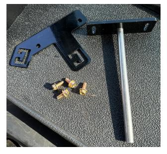
2. Attach the cable routing bracket (P/N 107-4001-093) to the DirecSteer assembly at the 10 o'clock position and tighten with two provided M5 x 12 bolts (P/N 311-4035-002K).
