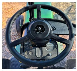
5. Install the included telescope locking knob (P/N 106-0159-783) on the telescope adapter (P/N 063-4001-058) and tighten the M8 nut and washer with a 13 mm socket.
