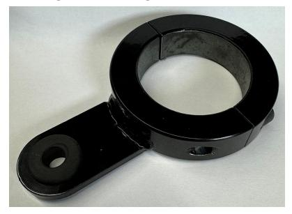
6. Attach the column clamp (P/N 116-4050-052) to the steering column with the grommet side pointing directly towards the operator seat. Secure with the provided hardware.
