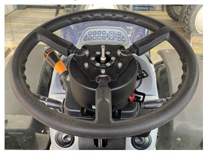
2. Remove the column nut and washer.
