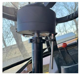
2. Secure the DirecSteer assembly to the steering column with the provided extended column nut (P/N 107-4001-157) and washer (P/N 313-2300-132). Tighten the nut to 54.25 Nm [40 ft\*lbs].
