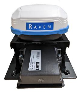
7. Attach the roof bracket (P/N 116-4001-001) to the RS1<sup>™</sup> fixed mount bracket (P/N 107-0172-498) with the provided four M6 x 16 countersink screws (P/N 311-4073-134) using a 4 mm hex key.
