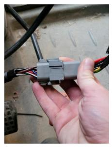
14. Connect the 18-pin connector of the field computer harness (P/N 115-7325-051/052) to the mating connector of the receiver tee cable (P/N 115-7325-021).
