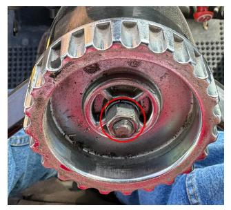
3. Bend down the tabs on the star-shaped washer to remove the column nut used to secure the steering wheel to the column.
