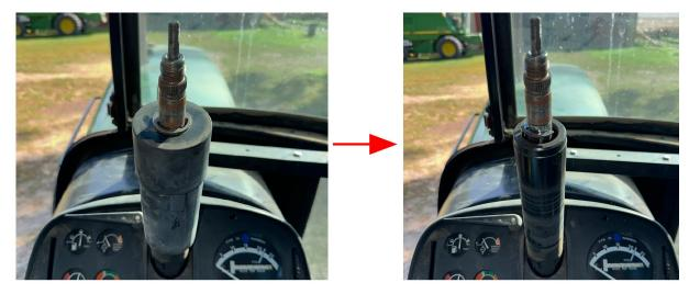
2. Fully thread the supplied telescope adapter (P/N 063-4001-082) on to the existing telescoping adjustment stem.
