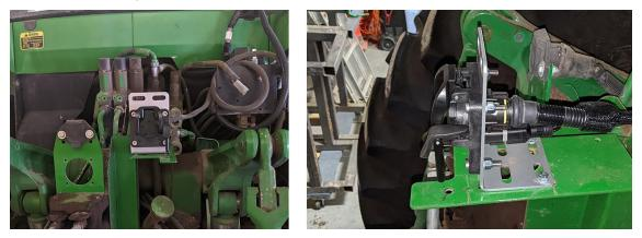
e. Connect the ISOBUS IBBC connector from the DirecSteer power harness (P/N 115-7325-012/013) to mounted IBBC connector.
