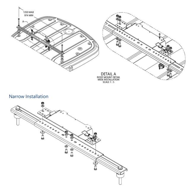
4. Install the bracket to the cab roof using the two 5/8-11 UNC x 3.5" bolts provided in the machine completion kit. It is not recommended to use the M16 x 130 bolts provided in the 117-5001-095 kit.
