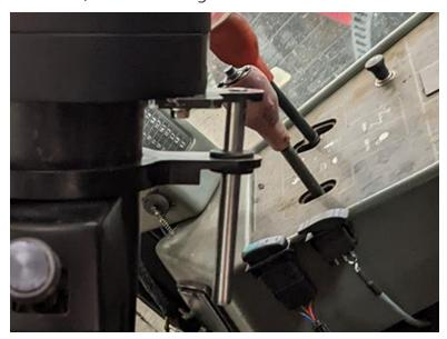
3. To keep the telescoping stem extended, use pliers or similar tool to grip and pull the previously installed bolt (P/N 311-0052-113) on the end of the telescoping stem.
