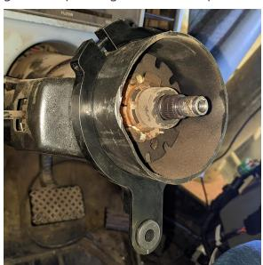
**Note:** The alignment of the column clamp may be further adjusted during installation. It is recommended to **not** fully tighten the hardware at this time.
