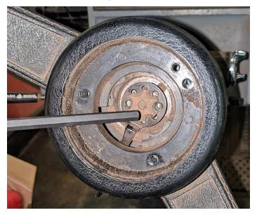
4. Remove the snap ring with retaining ring pliers with  $45^{\circ}$ ,  $.047^{\circ}$  tips.
