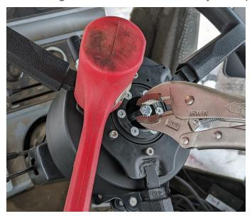
**Note:** It may be difficult to determine when the spline is fully mated. When correctly installed, the assembly should be stable and not wobble, and the threads on the steering column shaft should be exposed.
