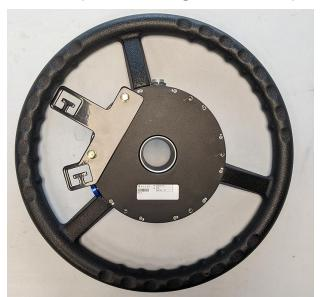
2. Attach the anti-rotation stem (P/N 063-4001-045) to the DirecSteer assembly at the 6 o'clock position with two of the provided bolts (P/N 311-4035-002K), but do not tighten.
