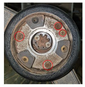
d. Remove the two hex screws with a 4 mm [5/32 in] hex wrench.
