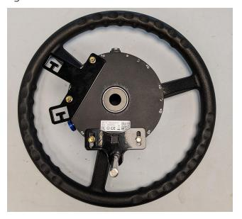
**Note:** The position of the anti-rotation stem may be further adjusted during installation. It is recommended to **not** fully tighten the bolts at this time.
