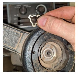
5. Remove the bolt with a 21 mm [7/8"] deep well socket.
