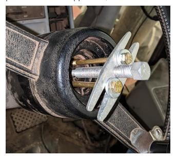
**Note:** An OEM Tools 27017 steering wheel puller with 1/4" -  $28 \times 4$ " grade 8 bolts is pictured above.
