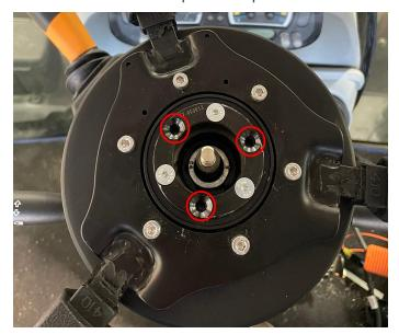
4. Attach an OTC 7403 steering wheel puller with M5  $\times$  0.8  $\times$  100+ mm bolts to the DirecSteer assembly. Use the provided spacer (P/N 305-1001-011) to protect the telescoping stem when applicable.
