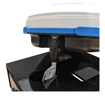
**Note:** It is easier to attach the connector before the antenna is attached to the roof bracket.
