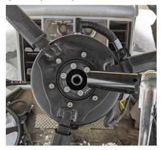
**Note:** If the nut and washer cannot be installed, make sure the spline adapter was correctly mated with the steering column by referencing the previous steps.
