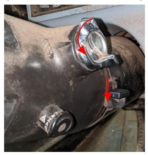
2. Remove the steering wheel cap:
