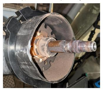
2. Insert the anti-rotation stem (P/N 063-4001-045) through the grommet in the flanged column clamp (P/N 107-4050-225) while also mating the spline adapter (P/N 107-4050-044) to the steering column.
