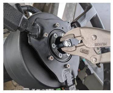
4. Pull back on the bolt and push down on the assembly until the spline is fully mated to the steering column. A rubber mallet may be helpful to fully mate the spline.
