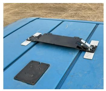
6. Attach and secure the antenna receiver onto the receiver bracket so that the antenna receiver is facing the front of the machine.
