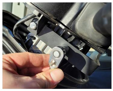
19. Pull up the rubber boot to the around the lower base of the column.
