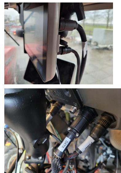
17. Once everything is installed and connected, hide the cabling behind the lining whenever possible, and tie down the cabling where appropriate to avoid loose cabling.
