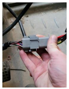
15. Connect the 18-pin connector of the field computer harness (P/N 115-7325-051/052) to the mating connector of the receiver tee cable (P/N 115-7325-021).
