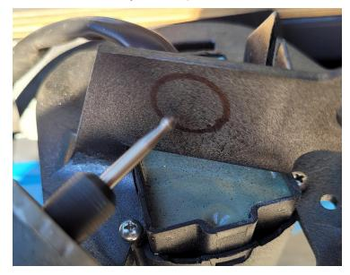
10. Attach the bolt cutout template (P/N 107-4050-121) to the opposite, smaller side of the cover using a bolt and nut in the existing mounting hole.
