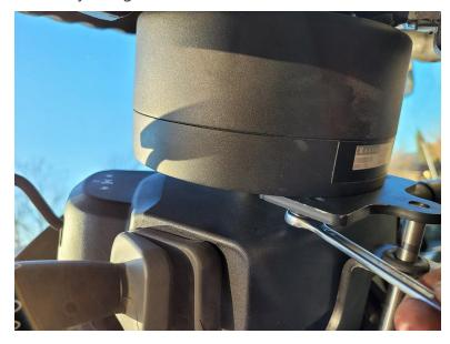
4. Install the cover over the center of the DirecSteer assembly.
