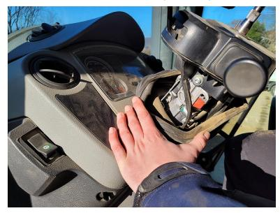
2. Remove the bolts securing the plastic base to the steering column using a T30 Torx screwdriver.
