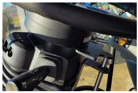
2. Install the original column nut and washer to the center of the assembly using a 22 mm socket.
