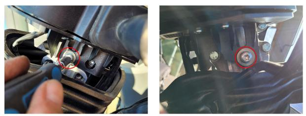
15. Remove the two bolts visible in the previously cut holes using a 10 mm socket.
