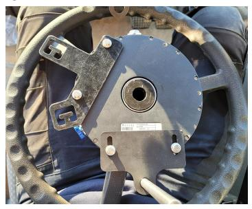
**Note:** The position of the anti-rotation stem may be further adjusted during installation. It is recommended to **not** tighten the bolts at this time.
