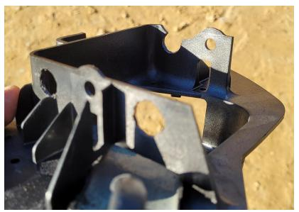
13. Reattach the top cover to the lever tray and insert the spline through the assembly.
