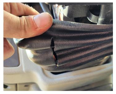
17. Insert the bolt-holes side of the grommet holder bracket (P/N 107-4001-191) through the slit in the rubber boot and along the left side of the steering column.
