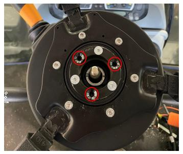
4. Attach an OTC 7403 steering wheel puller with M5 x 0.8 x 100+ mm bolts to the DirecSteer assembly. Use the provided spacer (P/N 305-1001-011) to protect the telescoping stem when applicable.
