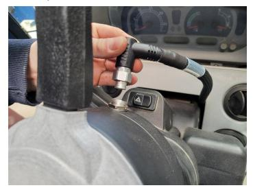
13. Route the DirecSteer motor cable (P/N 115-4001-258) along the wire routing bracket. Zip-tie the cabling as desired.
