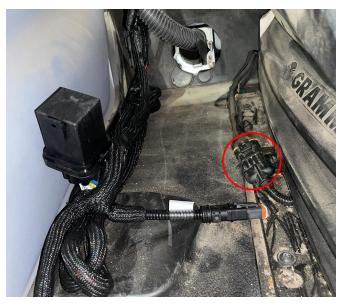
12. Connect motor cable (P/N 115-4001-258) to the electrical port on the DirecSteer assembly.
