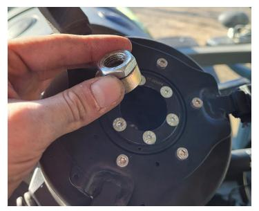
3. Tighten the two M5 x 12 bolts securing the anti-rotation stem to the DirecSteer assembly using a 8 mm wrench.
