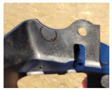
12. Cut out the hole with the Dremel rotary tool.
