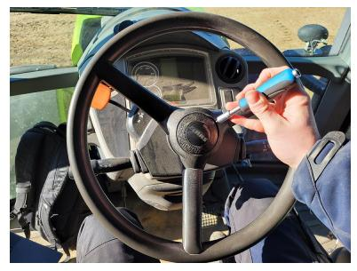
2. Remove the nut securing the steering wheel to the column with a 22 mm socket.
