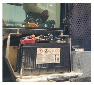
**Note:** Generally, the battery compartment is located on the right side of the tractor, in front of the rear tire and below or beside the tractor cab.
