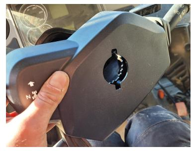
14. Reattach the base to the steering column using the original T30 Torx screws.
