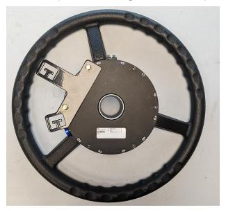
3. Attach the anti-rotation stem (P/N 063-4001-087) to the DirecSteer assembly at the 6 o'clock position with two of the provided bolts (P/N 311-4035-002K), but do not tighten.
