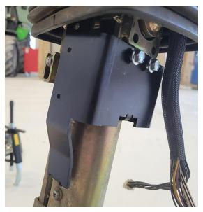
**Note:** The position of the anti-rotation bracket may be further adjusted during installation. It is recommended to **not** tighten the bolts at this time.
