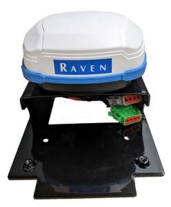
5. Connect the 12-pin DTM plugs on the 500S<sup>™</sup>/SC1<sup>™</sup> cable to the mating connectors on the SC1<sup>™</sup>/TC1<sup>™</sup> unit.
