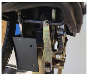
33. Place the retainers back on the pins using a small flat-head screwdriver.
