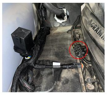
12. Connect motor cable (P/N 115-4001-258) to the electrical port on the DirecSteer assembly.
