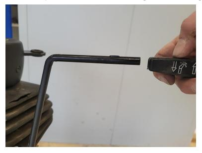
23. Pull up on the steering column locking lever and push the small edge out of the latch.
