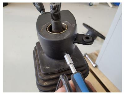
7. Lift up the steering column up from the dashboard to expose the lower plastic covers.
