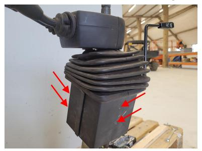
9. Pull the rubber boot upwards to expose the black inner bracket.
