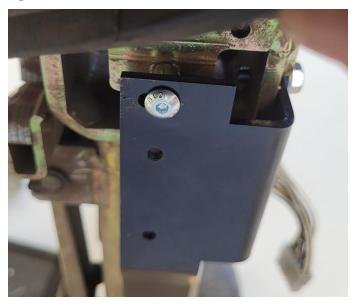
18. Push the bracket so that the flange head bolts are fully pressed against the left side of the slot.
