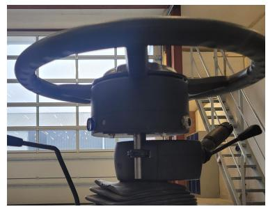
2. Fully tighten the anti-rotation stem hardware.
