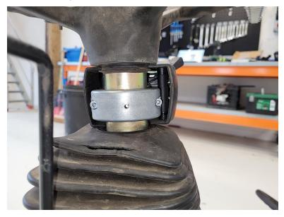
3. Mark the existing clamp position of the switch assembly on the steering column.
