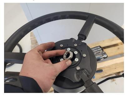
4. Install the cover over the center of the DirecSteer assembly.
