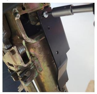
21. Remove the two retainers from the steering column locking lever using a small flathead screwdriver.
