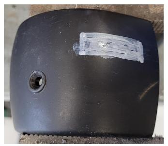
5. Use a Dremel rotary tool to cut out the rectangle slot.
