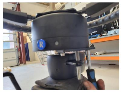
3. Install the original column nut to the center of the assembly using a 27 mm socket.
