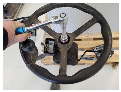
8. Use a steering wheel puller to remove the steering wheel from the spline shaft.
