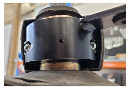
2. Attach the cutout template (P/N 107-4001-192) to the outside of the plastic cover and secure using the previously removed screw on the outside and the previously removed clamp on the inside of the cover.
