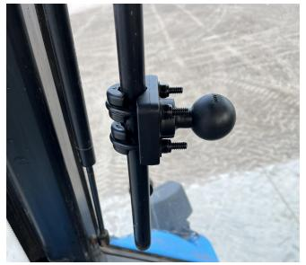
c. If provided with mounting bracket (P/N 107-8000-082) and the machine has a matching bolt pattern, the display mount can be attached to a cab post.
