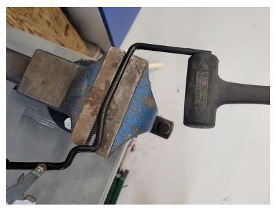
31. Verify the 58° angle using a protractor.
