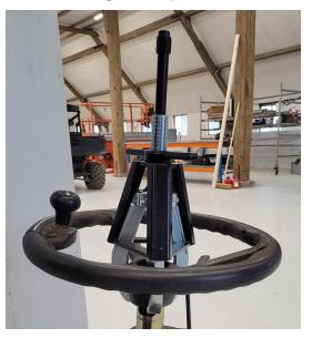
**Note:** A Posi-Lock model 106 steering wheel puller is recommended.
