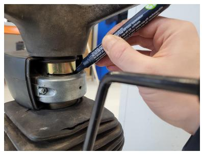
4. Remove the screws securing the clamp to the steering column using a 4 mm Allen key.
