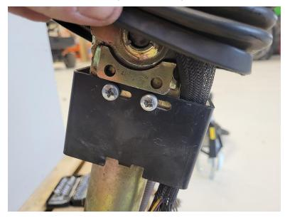
10. Remove the black inner bracket by unscrewing the two screws using a #3 Phillips head screwdriver.
