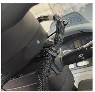
14. Route the 8-pin connector of the DirecSteer motor cable (P/N 115-4001-258) to the mating connector labeled "DirecSteer Motor Cable" on the DirecSteer main cable (P/N 115-7325-021).
