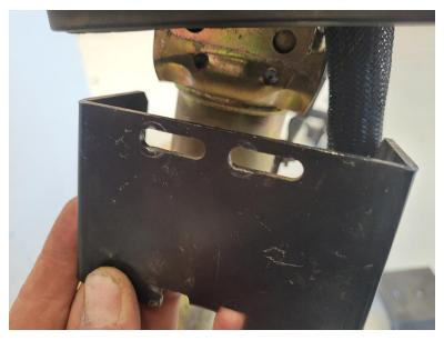
11. Check to see if the steering column can be easily rotated by hand. Rotation or movement of the steering column after the DirecSteer installation will decrease the steering accuracy.
