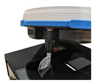
**Note:** It is easier to attach the connector before the antenna is attached to the roof bracket.
