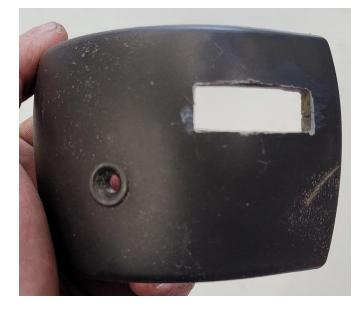
6. Attach the cover to the column while inserting the grommet through the slit. Secure with the previously removed 4 mm screw using a #2 Phillips head screwdriver.
