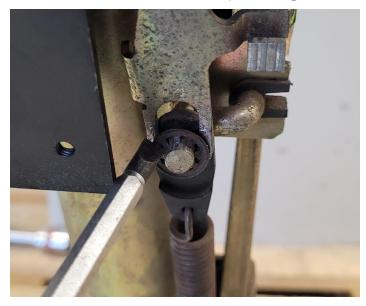
34. Attach the plastic handle back onto the column locking lever.
