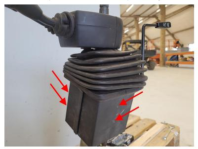
35. Reinstall the plastic covers with the previously removed #2 Phillips screws.
