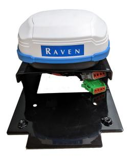
5. Connect the 12-pin DTM plugs on the 500S™/SC1™ cable to the mating connectors on the SC1™/TC1™ unit.
