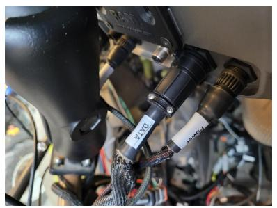
17. Once everything is installed and connected, hide the cabling behind the lining whenever possible, and tie down the cabling where appropriate to avoid loose cabling.
