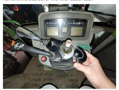
3. Remove two socket head bolts from the clamp holding the wiper levers with a 4 mm Allen wrench to remove the clamp.
