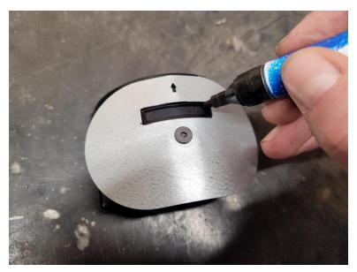
7. Use a Dremel to cut the hole out of the cover.
