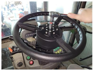
3. Tighten the anti-rotation stem (P/N 063-4001-084) bolts with a 8 mm wrench or socket.
