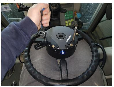
**Note:** The position of the anti-rotation stem may be further adjusted during installation. It is recommended to **not** tighten the bolts at this time.
