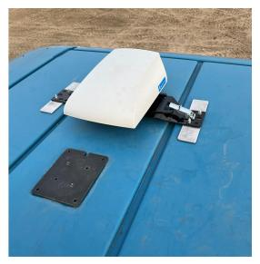
7. If applicable, mount the round adhesive plate for the LAIRD cellular antenna (P/N 121-0000-042) within 50 cm [20 in] from the antenna receiver bracket.
