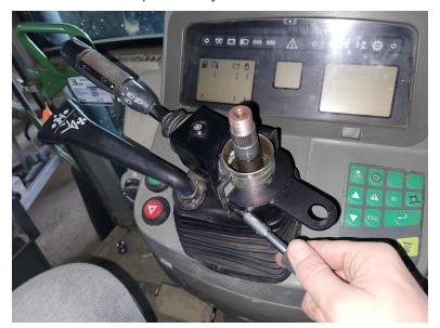
5. Install the provided template (P/N 107-4001-179) to the outside of the plastic cover as shown, use the original clamp and the supplied M4x12 counter head screw (P/N 311-4070-047K).
