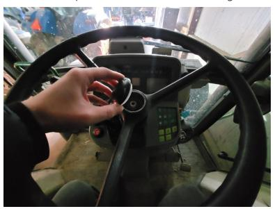
2. Remove the large nut securing the steering wheel with a 27 mm socket.
