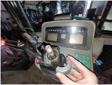
4. Mount the anti-rotation clamp (P/N 116-4050-012) to the steering column using the screws that were previously removed.
