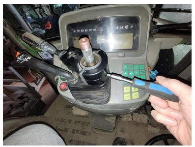
2. Remove the side cover with the rubber seal.
