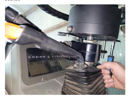
4. Install the cover (P/N 106-0159-782) over the center of the DirecSteer steering wheel.
