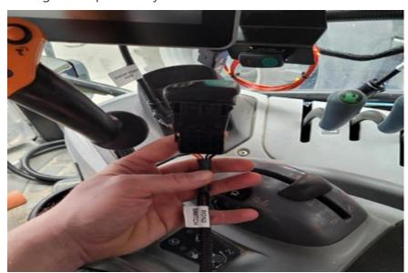
9. Press the switch assembly into the cavity to seat the switch.
