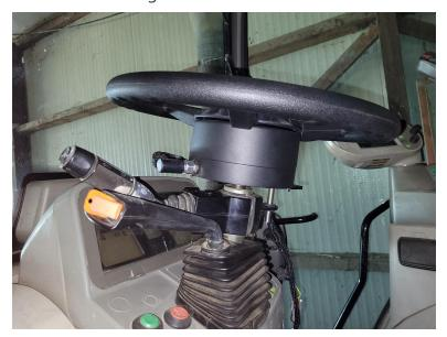
2. Install the flanged column nut (P/N 312-1001-202) in the spline adapter and tighten with a 24 mm deep socket.
