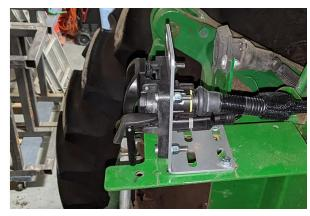
e. Connect the ISOBUS IBBC connector from the DirecSteer power harness (P/N 115-7325-012/013) to mounted IBBC connector.
