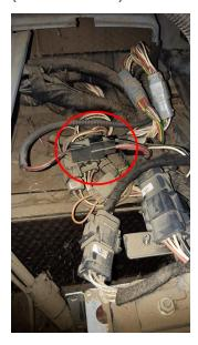
12. Connect motor cable (P/N 115-4001-258) to the electrical port on the DirecSteer assembly.
