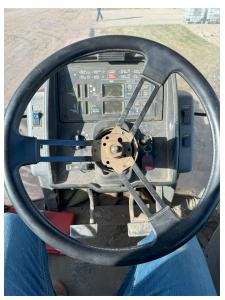
5. Use a 1 1/4" or 32 mm deep well socket to remove the large nut securing the steering wheel.
