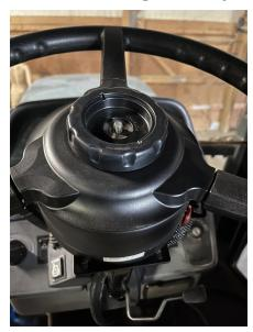
7. Secure the adjustable knob with M8 washer and nylock nut.
