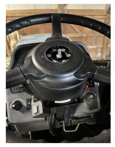
6. Install the steering wheel adjustable knob (P/N 106-0159-784).
