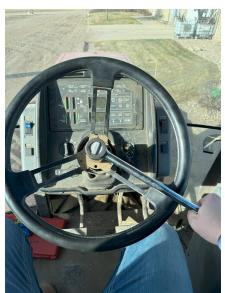
6. Use a Phillips screwdriver to remove the three screws in the steering wheel hub.
