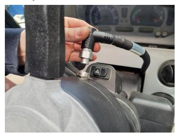
14. Route the DirecSteer motor cable (P/N 115-4001-258) along the wire routing bracket. Zip-tie the cabling as desired.
