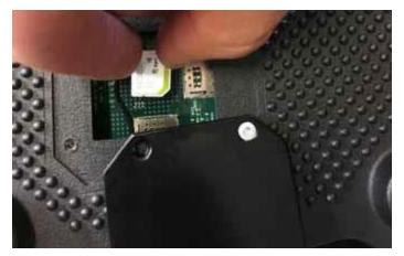
**Note:** The SIM card must be inserted into the J11 slot or the RS1<sup>TM</sup> will not connect to wireless or a CORS network.
