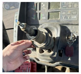
3. Push down the rubber boot until the metal column is fully visible.
