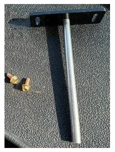
2. Attach the cable routing bracket (P/N 107-4001-093) to the DirecSteer assembly at the 10 o'clock position and tighten with two provided M5 x 12 bolts (P/N 311-4035-002K).
