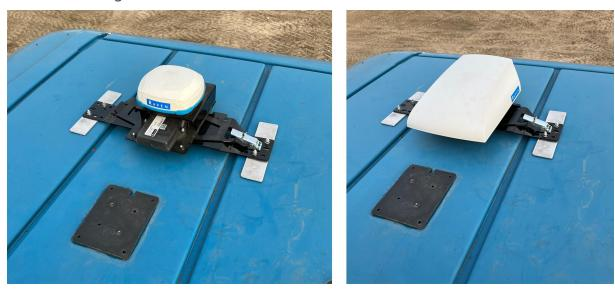
7. If applicable, mount the round adhesive plate for the LAIRD cellular antenna (P/N 121-0000-042) within 50 cm [20 in] from the antenna receiver bracket.
