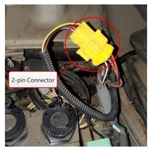
12. Attach the seat switch tee (P/N 115-7325-070) to the 2-pin operator presence connector on the cabin cable (P/N 115-7325-021) and tee into the 2-pin seat cable (circled below).
