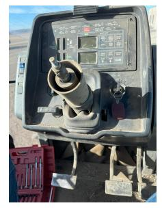
2. Remove the lower tube cover and the plastic ring.
