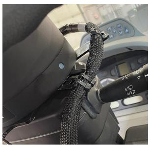
15. Route the 8-pin connector of the DirecSteer motor cable (P/N 115-4001-258) to the mating connector labeled "DirecSteer Motor Cable" on the DirecSteer main cable (P/N 115-7325-021).
