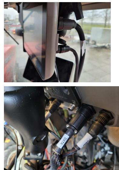
18. Once everything is installed and connected, hide the cabling behind the lining whenever possible, and tie down the cabling where appropriate to avoid loose cabling.
