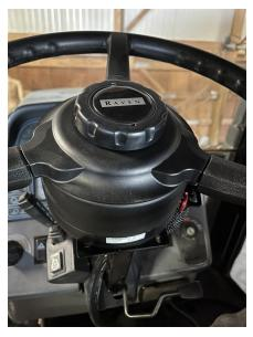
9. Check that all hardware is properly tightened and the DirecSteer is secure.
