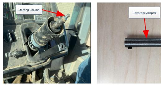
2. Install the DirecSteer assembly on the steering column.
