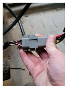
16. Connect the 18-pin connector of the field computer harness (P/N 115-7325-051/052) to the mating connector of the receiver tee cable (P/N 115-7325-021).
