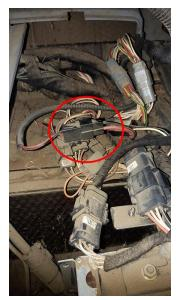
13. Connect motor cable (P/N 115-4001-258) to the electrical port on the DirecSteer assembly.
