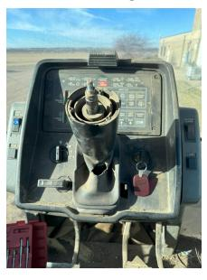
**Note:** The factory steering wheel and components will not be used with the DirecSteer system. It is recommended to keep these components in case the DirecSteer system will be uninstalled or moved to a different machine.
