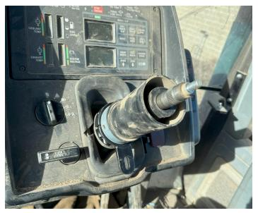
8. Loosely install the grommet holder weldment (P/N 116-4050-065) with the M8-1.25x20 mm hex flanged bolt (P/N 311-4035-054K).
