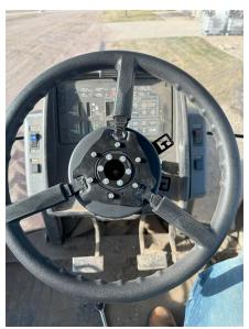
5. Install the cover (P/N 106-0159-781) to the center of the DirecSteer steering wheel.
