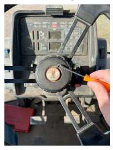
3. Use a 9/16" or 14 mm deep well socket to remove the nut used to secure telescope locking mechanism to the steering column.
