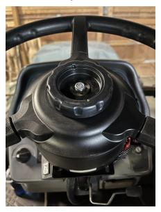
8. Install the cover of the knob on the steering wheel.
