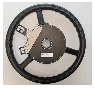
3. Attach the anti-rotation stem (P/N 063-4001-073) to the DirecSteer assembly at the 6 o'clock position with two of the provided bolts (P/N 311-4035-002K), but do not tighten.
