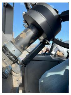
4. Secure the DirecSteer assembly to the steering column using the extended column nut (P/N 107-4001-162) and M20 washer (P/N 313-6000-131K).
