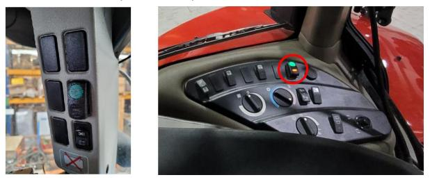
**Note:** If needed, use the supplied switch adapter (P/N 412-8000-037) when installing in a larger sized cavity.
