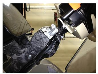
11. Use the previously removed screws to secure the two plastic steering angle covers together, and align the top edge of the joined covers with the top edge of the cutout template (P/N 107-4001-196).
