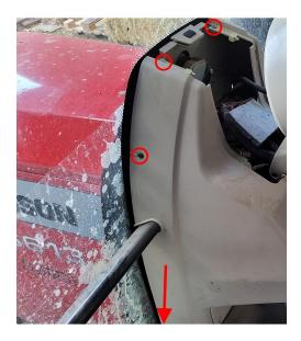
**Note:** There are two screws on the opposite side of the steering column.
