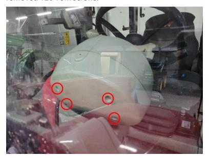
18. Reinstall the five previously removed screws behind the foot pedals.
