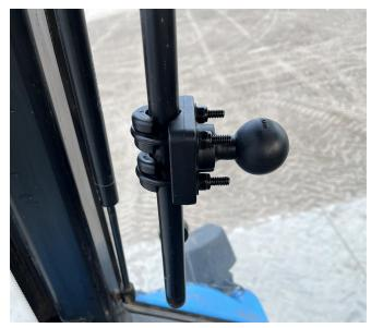
c. If provided with mounting bracket (P/N 107-8000-082) and the machine has a matching bolt pattern, the display mount can be attached to a cab post.
