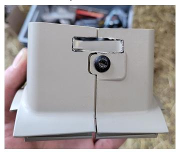
14. Install the anti-rotation bracket clamp (P/N 107-4050-135) on the top of the steering column.
