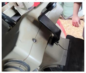
16. Reinstall the side panels by securing with the six previously removed screws.
