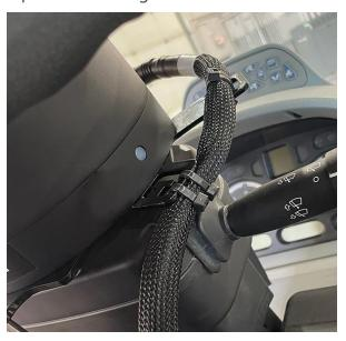
14. Route the 8-pin connector of the DirecSteer motor cable (P/N 115-4001-258) to the mating connector labeled "DirecSteer Motor Cable" on the DirecSteer main cable (P/N 115-7325-021).
