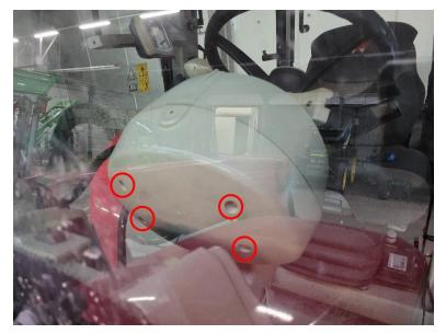
8. Remove the back cover of the instrument panel.
