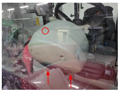
**Note:** Two screws are located on the bottom of the panel.
