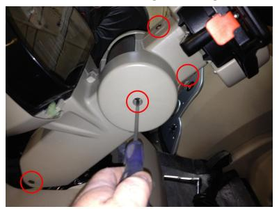
**Note:** There are two screws on the opposite side of the steering column.
