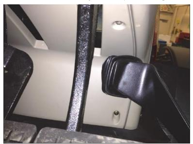
7. Remove the four screws behind the instrument cluster using a T20 Torx screwdriver.
