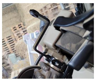
15. Reinstall the steering angle covers to the steering column.
