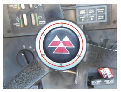
2. Remove the nut securing the original steering wheel to the column with a 22 mm socket.
