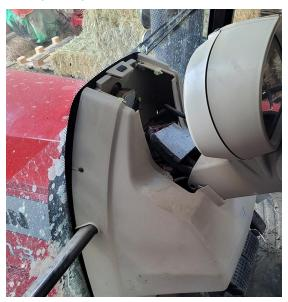
5. Remove the two screws on the top, two screws on the left side, and two screws on the right side of the dashboard cover using a T20 Torx screwdriver.
