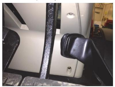
19. Reinstall the six previously removed screws on the top and the sides of the back dashboard covers.
