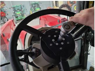
3. Tighten the two M5  $\times$  12 bolts to secure the anti-rotation stem with a 8 mm wrench.
