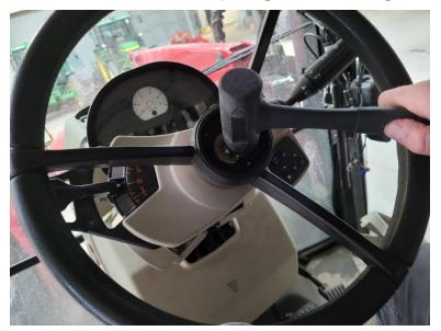
**Note:** The factory steering wheel and components will not be used with the DirecSteer system. It is recommended to keep these components in case the DirecSteer system will be uninstalled or moved to a different machine.
