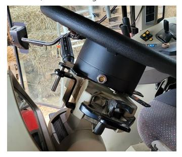
2. Insert the original column nut, washer, and two additional washers in the spline adapter and tighten.
