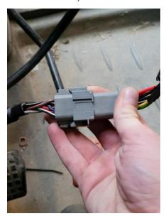
15. Connect the 18-pin connector of the field computer harness (P/N 115-7325-051/052) to the mating connector of the receiver tee cable (P/N 115-7325-021).
