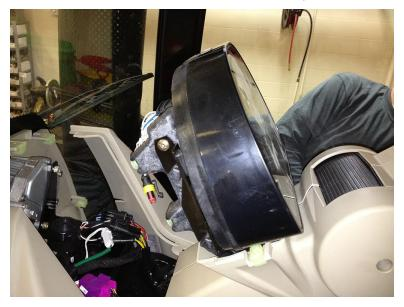
9. Remove the six screws securing the steering column covers.
