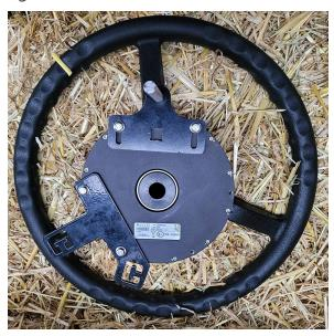
**Note:** The position of the anti-rotation stem may be further adjusted during installation. It is recommended to **not** tighten the bolts at this time.
