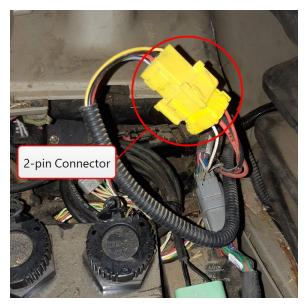
12. Connect motor cable (P/N 115-4001-258) to the electrical port on the DirecSteer assembly.
