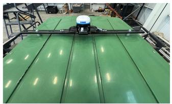
6. If applicable, mount the round adhesive plate for the LAIRD cellular antenna (P/N 121-0000-042) within 50 cm [20 in] from the antenna receiver bracket.
