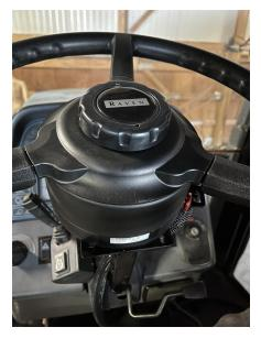
11. Check that all hardware is properly tightened and the DirecSteer is secure.
