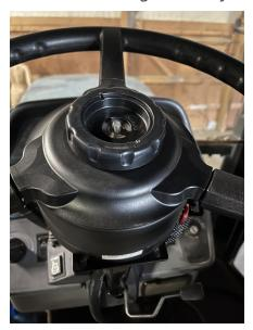
9. Secure the adjustable knob with M8 washer and nylock nut.
