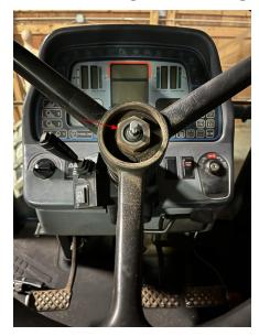
5. Install the spacer (P/N 305-1001-011) to protect the telescoping stem.
