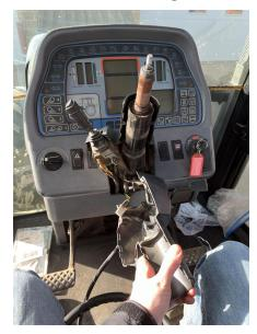
7. Tilt the steering column down and remove the front cover.
