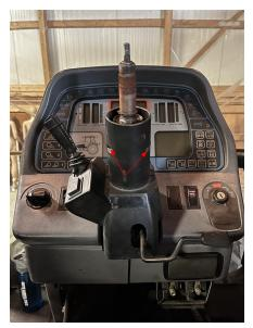
4. Remove the two screws from the lower part of the steering column cover.
