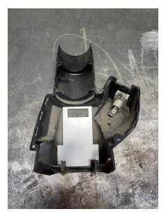
9. Cut the opening in the steering wheel column cover with a Dremel rotary tool equipped with a cutting disk (EzCut 426/456 recommended) and multipurpose cutting bit (561 recommended).
