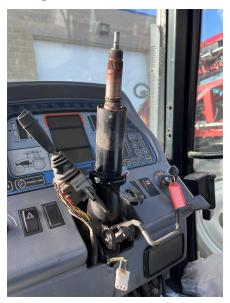
13. Tighten the flanged column clamp to the steering column.
