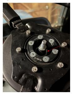
7. Install the cover (P/N 106-0159-781) to the center of the DirecSteer steering wheel.
