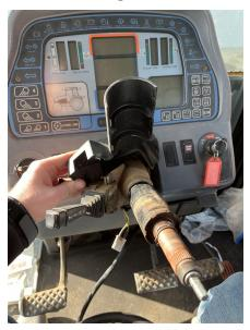
8. Install the supplied template (P/N 107-4001-154) as a guide. Mark the area to be removed.
