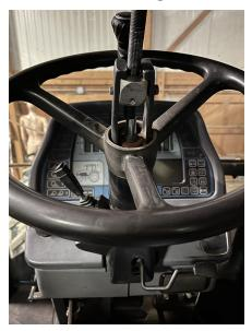
**Note:** The factory steering wheel and components will not be used with the DirecSteer system. It is recommended to keep these components in case the DirecSteer system will be uninstalled or moved to a different machine.
