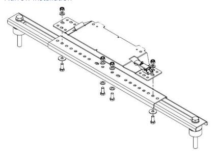
4. Install the bracket to the cab roof using the two M16  $\times$  100 bolts provided in the machine completion kit. It is not recommended to use the M16  $\times$  130 bolts provided in the 117-5001-095 kit.
