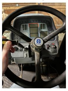
2. Remove the nut used to secure telescope locking mechanism to the steering column with a 13 mm socket.
