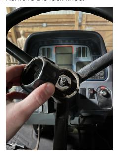
4. Remove the large nut securing the steering wheel.
