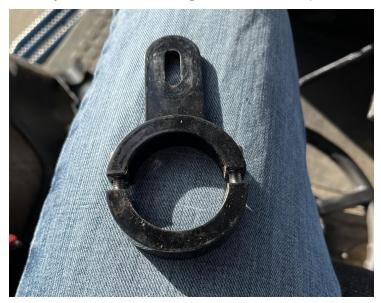
12. Slide the assembled flanged column clamp over the steering column with the flat side facing down.
