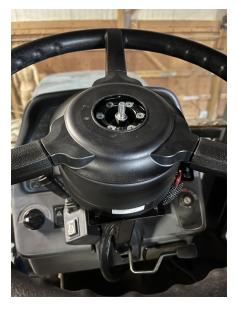
8. Install the steering wheel adjustable knob (P/N 106-0159-784).
