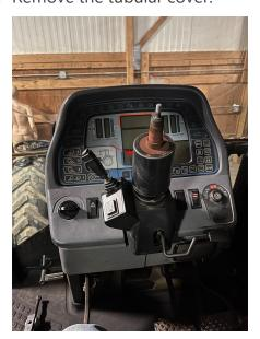
3. Remove the two screws from the top of the steering column cover.
