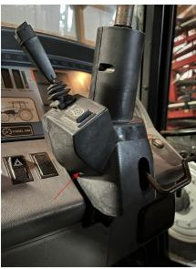
5. If necessary disconnect the ether switch connector.
