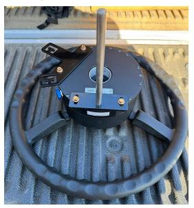
**Note:** The position of the anti-rotation stem may be further adjusted during installation. It is recommended to **not** tighten the bolts at this time.
