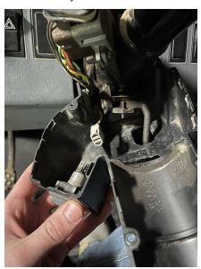
6. Slide the rear steering column cover over the tilt lever.
