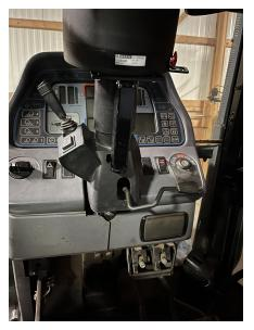
5. Secure the DirecSteer assembly to the steering column using the extended column nut (P/N 107-4001-162) and M20 washer (P/N 313-6000-131K).
