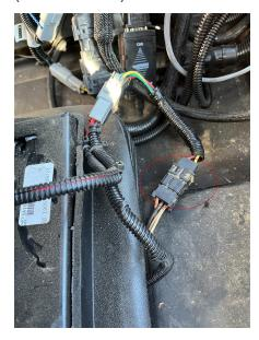
12. Connect motor cable (P/N 115-4001-258) to the electrical port on the DirecSteer assembly.
