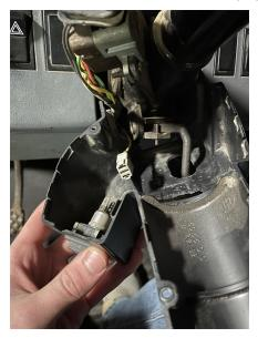
16. Tilt the steering column half way up install the modified cover. The modified cover should snap into the front cover.
