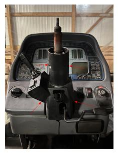
18. Install the tubular cover over the steering shaft.
