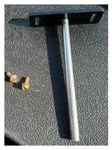
2. Attach the cable routing bracket (P/N 107-4001-093) to the DirecSteer assembly at the 10 o'clock position and tighten with two provided M5 x 12 bolts (P/N 311-4035-002K).
