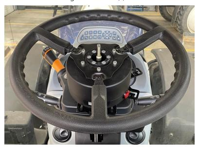
2. Remove the column nut and washer.
