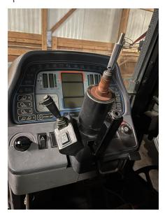
3. Install the DirecSteer assembly on the steering column.
