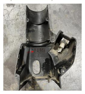
10. Use a file to clean the edges of the holes to ensure there are no burrs or sharp surfaces.
