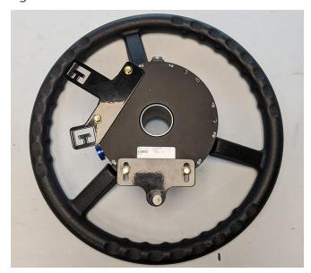
**Note:** The position of the anti-rotation stem may be further adjusted during installation. It is recommended to **not** tighten the bolts at this time.
