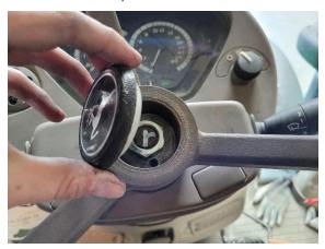
2. Use a 27 mm socket to remove the nut.
