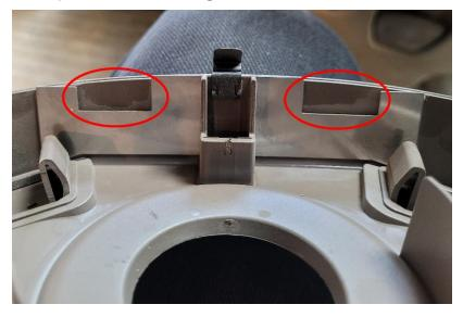
28. Insert the supplied spacers (P/N 107-4050-161) on the screw holes as shown below.
