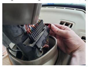
8. Slide the remaining mounted part of the connector out of its mount.
