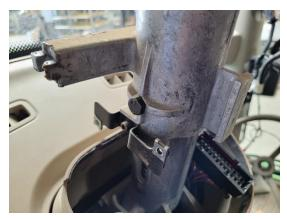
14. Thread one of the M6  $\times$  20 mm bolts and washer in the anti-rotation block (P/N 107-4050-163).
