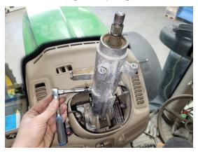
19. After tightening, remove the lower bolt.
