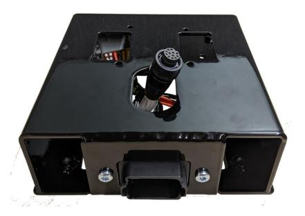
3. Connect the 12-pin circular connector to the 500S<sup>™</sup> receiver (P/N 063-2000-006/-013).
