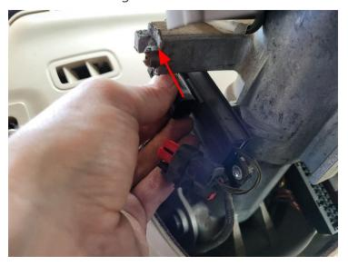
11. Lift the instrument cluster off the steering column.
