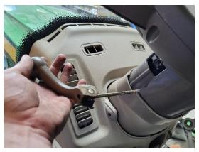
4. Tilt the steering column fully upwards.
