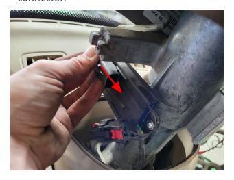
23. Connect the previously removed connectors together on both sides and ensure all the connectors are latched shut.
