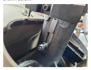
17. Press down on the steering column and align the top hole in the block with the hole in the side of the steering column.
