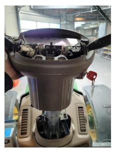
22. Slide the male connectors back into the mounting brackets.
