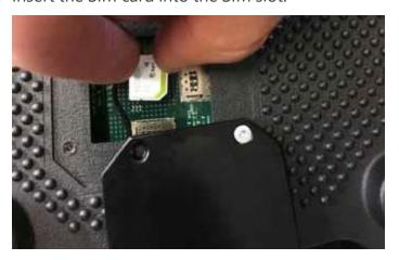
**Note:** The SIM card must be inserted into the J11 slot or the RS1<sup>m</sup> will not connect to wireless or a CORS network.
