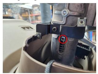
20. If applicable, remount the connector holder on the left side of the column using a Philips head screwdriver.
