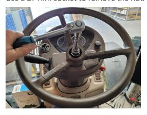
3. Pull upwards on the steering wheel to take it of its spline. If it doesn't come off by hand, use a steering wheel puller.
