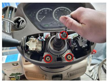
3. Remove the telescope locking lever using a 5 mm hex key.
