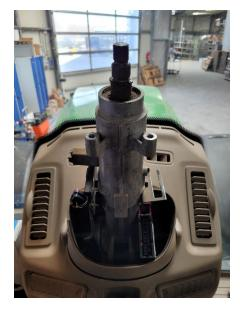
12. If applicable, remove the plastic connector mount from the steering column by removing the two screws with a small Philips head screwdriver.
