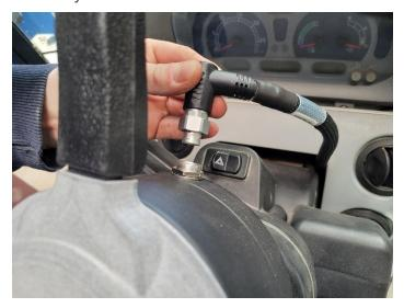
13. Route the DirecSteer motor cable (P/N 115-4001-258) along the wire routing bracket. Zip-tie the cabling as desired.
