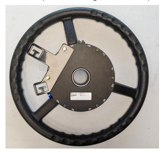
3. Attach the anti-rotation stem (P/N 063-4001-075) to the DirecSteer assembly at the 6 o'clock position with two of the provided bolts (P/N 311-4035-002K), but do not tighten.
