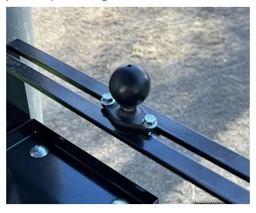
c. Attach the RAM® Mount to any rigid vertical or horizontal surface capable of supporting the weight of the field computer.
