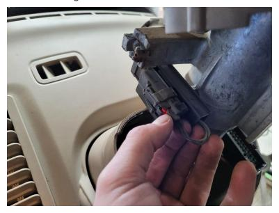
10. Press the black latch and pull the connectors apart. After separating the connectors, slide the remaining connector backwards to remove it.
