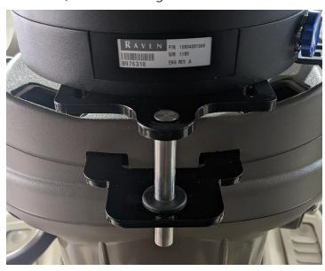
2. Insert the M18 washer (P/N 313-6000-028K) and column nut (P/N 107-4001-111) in the spline adapter and tighten with a 22 mm deep well socket.
