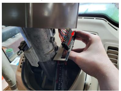
**Note:** Some John Deere machines may have this same kind of connector on the left side of the steering column. Remove that connector in the same manner as this connector.
