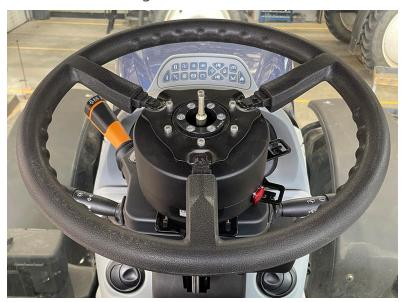
2. Remove the column nut and washer.
