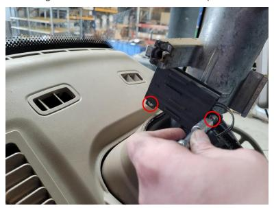
13. Remove the M8 bolt on the left side of the steering column with a 13 mm socket.
