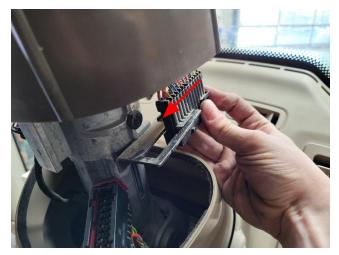
**Note:** Some John Deere machines may have this same kind of connector on the left side of the steering column. Reattach that connector in the same manner as this connector.
