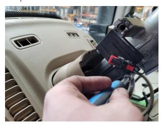
21. Make sure the steering column is fully extended again for easier installation. Put the instrument cluster back over the column and let it rest on the top part of the steering column so the connector mounts don't get covered.
