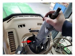
18. Insert the supplied M6x20mm bolt in the threaded hole of the column and tighten it down, securing the spring tensioner to the top part of the steering column.
