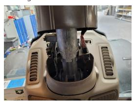
7. Disconnect the connector with the purple locking mechanism by pulling out the wedge. If the wedge is hard to remove, try prying it open with a flat-head screwdriver.
