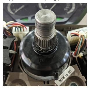
6. Lift up the complete dashboard and lean it on top of the column inside the plastic housing to reveal the connectors.
