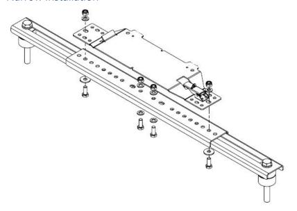
4. Install the bracket to the cab roof using the two M16 x 130 bolts provided in the machine completion kit.
