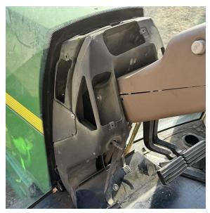
3. Remove the two screws from the upper steering column cover.
