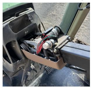
**Note:** The cold start button may need to be pushed in to remove the cover.
