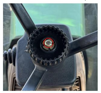
3. Remove the telescope locking mechanism and washer.
