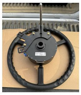
2. Secure with three of the provided bolts (P/N 311-4035-002K) but do not tighten.
