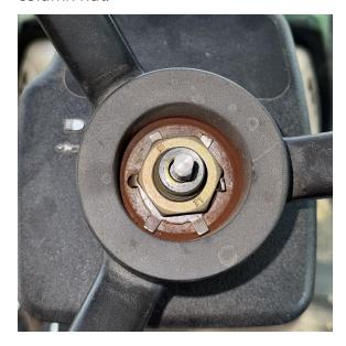
5. Remove the steering column nut.
