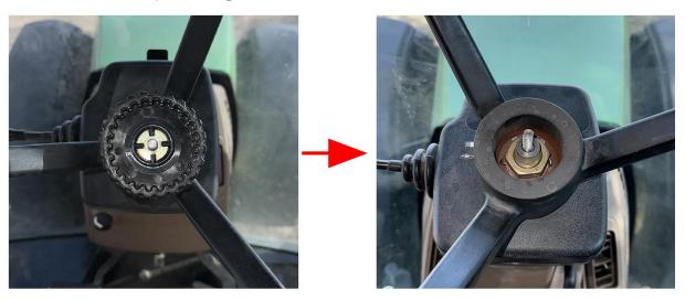
4. Bend down the lips of the nut retainer with a screwdriver to get access to the steering column nut.
