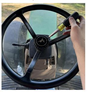
2. Remove the nut used to secure telescope locking mechanism to the steering column.
