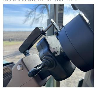
4. Install the extended column nut (P/N 107-4001-180) and M20 washer (P/N 313-6000-131K) over the telescope adapter (P/N 063-4001-259). Torque the nut to 45-54 Nm [33-40 ft lbs.].
