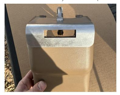
10. Place the top cover back on the steering column with the top of the anti-rotation bracket inserted through the cutout.
