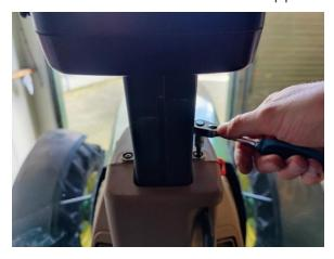
4. Remove the top cover from the steering column.
