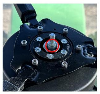
5. If installing on a 7XXX series machine, attach the E clip (P/N 335-0000-338) to the bottom of the anti-rotation stem.
