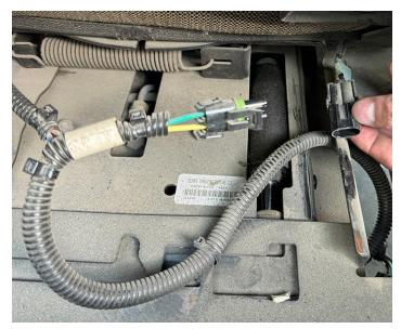
12. Connect motor cable (P/N 115-4001-258) to the electrical port on the DirecSteer assembly.
