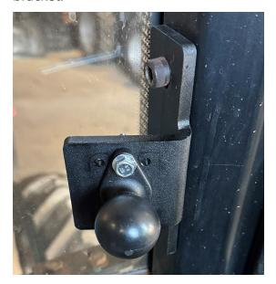
b. Attach the RAM® Mount to the John Deere display bracket. Use the silver backer plate to span the larger center slot of the bracket.
