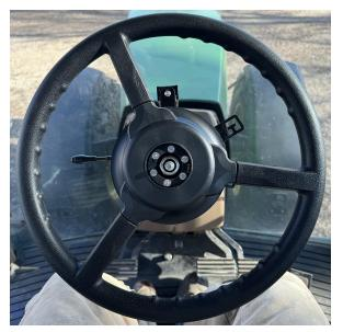
7. Install the telescope locking knob (P/N 106-0159-783) on the telescope adapter (P/N 063-4001-259) and tighten the M8 nut with the M8 washer (P/N 313-6000-013K).
