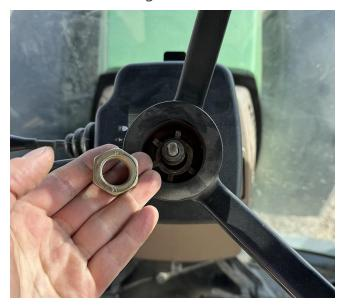
6. Remove the steering wheel by hand. If needed, use a steering wheel puller to remove the steering wheel.
