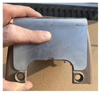
8. If needed, use a clamp to hold the cutout template in place.
