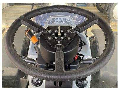
2. Remove the column nut and washer.
