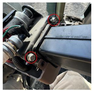
6. Place the holes of the anti-rotation bracket (P/N 107-4050-117) over the bolt-holes and secure with the supplied M6 x 25 bolts (P/N 311-4035-030K).
