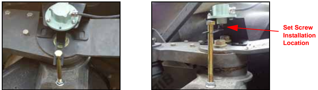
FIGURE 3. Rotary Sensor Installed
