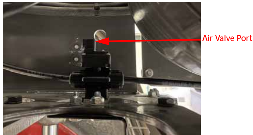
FIGURE 26. Valve Air Line Connections
