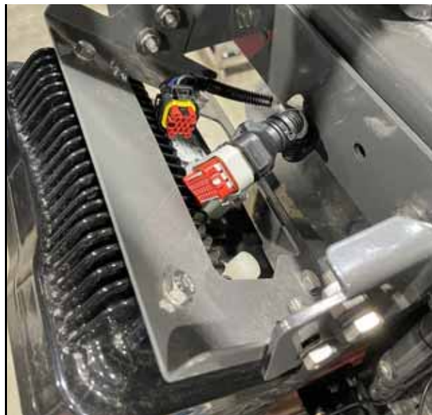
FIGURE 31. Connect to Ports on Rear of VSN
