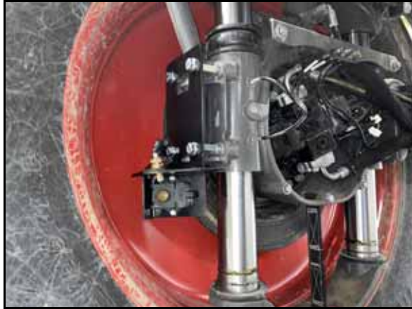
FIGURE 7. Radar Sensor Bracket Mounted
