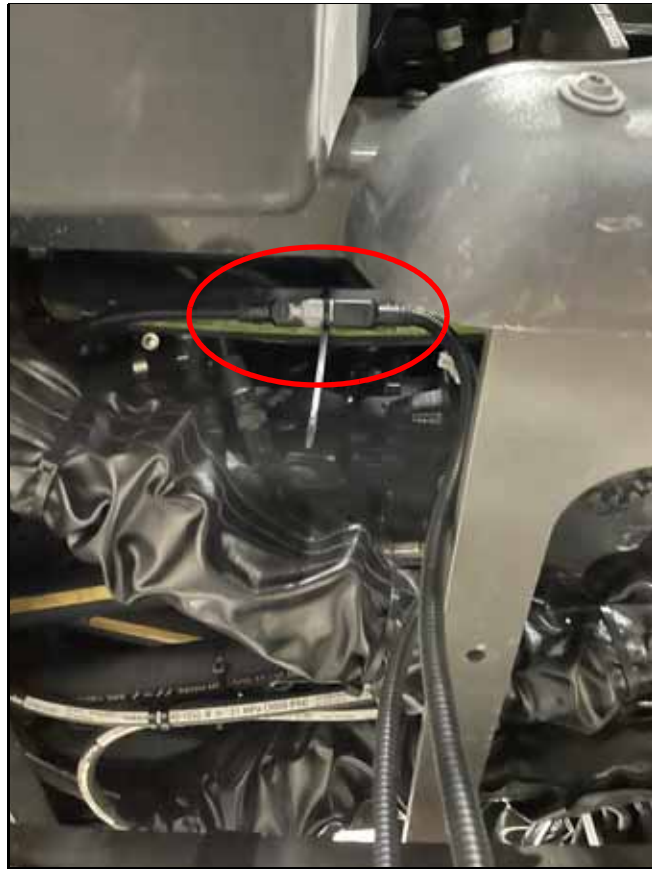
FIGURE 29. Valve Air Line Connections
