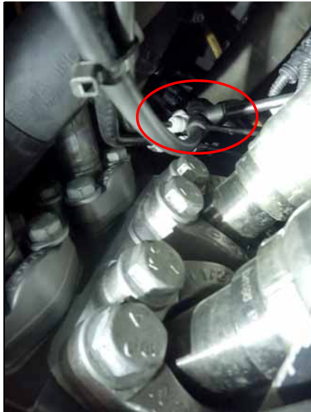
FIGURE 22. Install and Connect Air Tee
