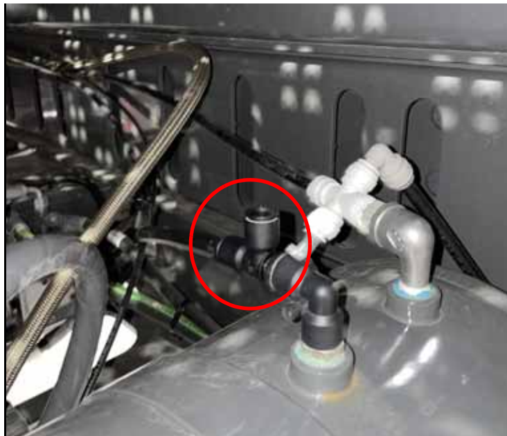
FIGURE 17. Install Run-Tee Fitting
