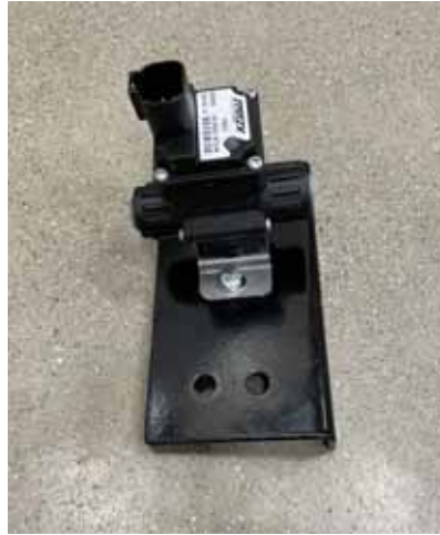
FIGURE 14. Assemble Air Valve and Mounting Brackets
