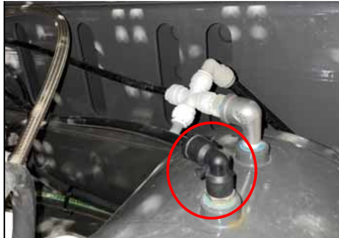
FIGURE 16. Factory Air 90° Elbow Fitting
