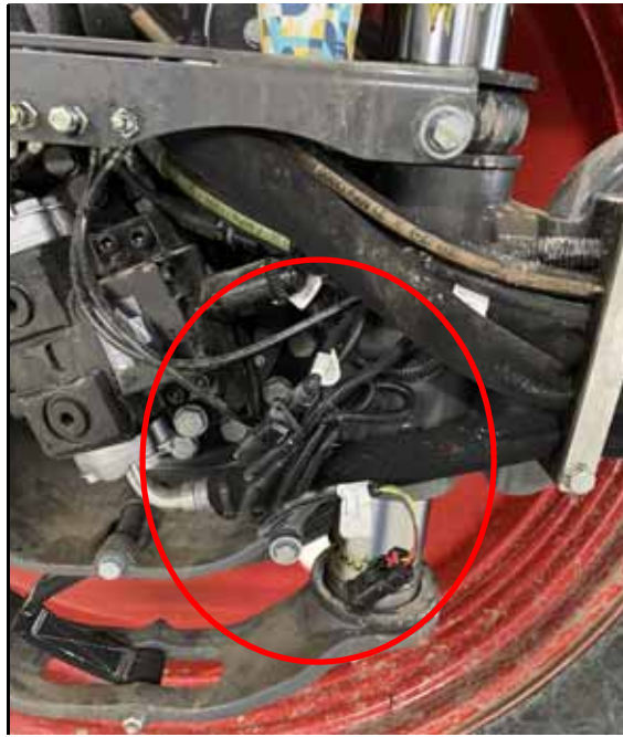
FIGURE 8. Factory Provisioned Radar Sensor Harness
