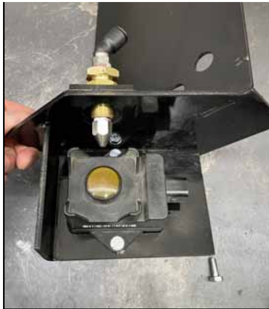
FIGURE 1. Radar Sensor Mounted to Bracket
