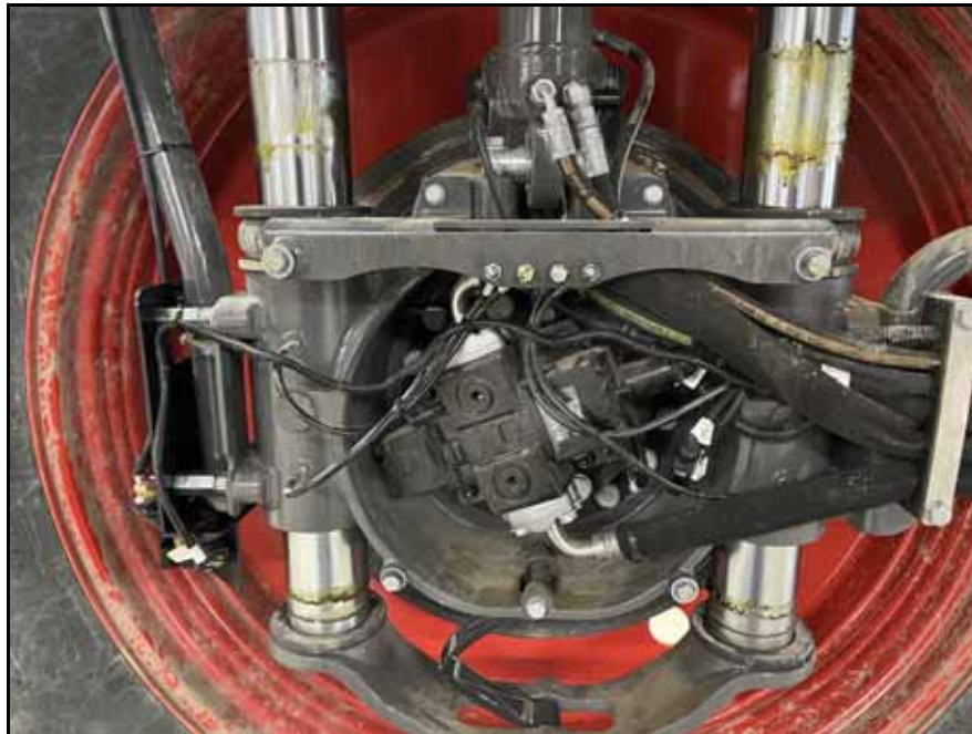
FIGURE 9. Connect Radar Sensor Harness
