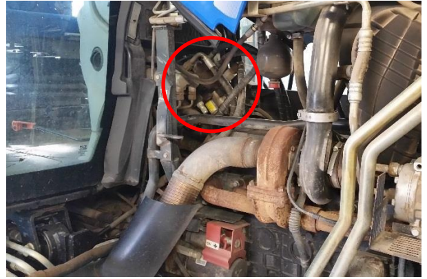
FIGURE 2 LOCATION CNH STEERING VALVE
