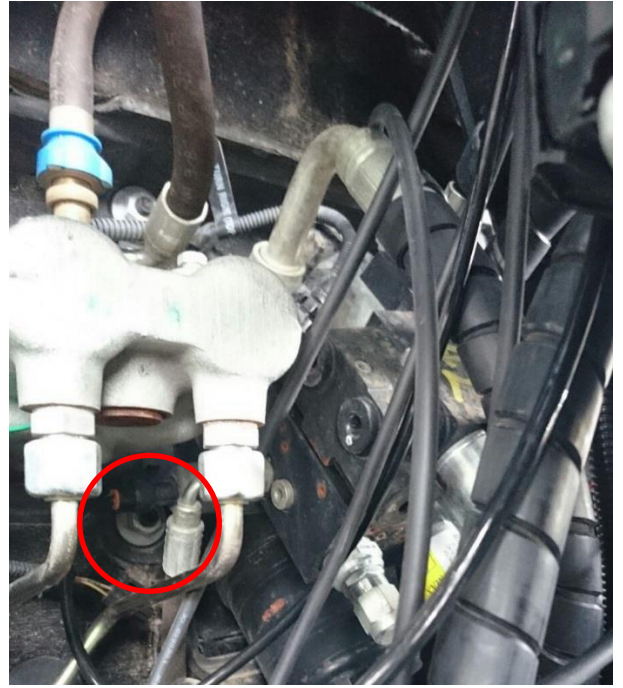
FIGURE 5 CONNECTION OF THE HDU – NH INTELLISTEER HARNESS ON THE CNH PRESSURE SENSOR
