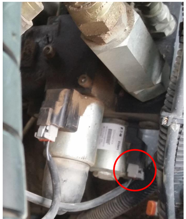
FIGURE 4 CONNECTION OF THE HDU – NH INTELLISTEER HARNESS ON THE CNH LOCK VALVE
