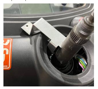
15. Mark the location directly under the small hole on the template.
