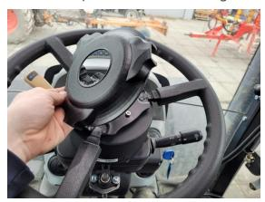
7. Place the telescope locking knob followed by M8 washer on the threaded rod.
