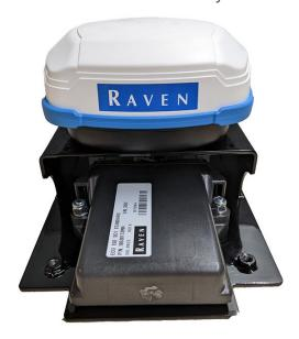
7. Attach the roof bracket (P/N 116-4001-001) to the RS1 $^{\text{m}}$  fixed mount bracket (P/N 107-0172-498) with the provided four M6 x 16 countersink screws (P/N 311-4073-134) using a 4 mm hex key.
