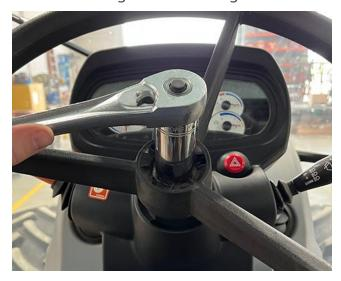
5. Remove the steering wheel using a steering wheel puller and M6x1.0 bolts. Use the provided spacer (P/N 305-1001-011) to protect the telescoping stem during removal.
