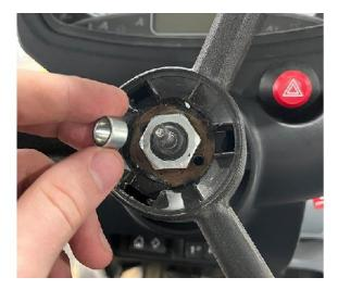
4. Remove the larger hex nut using a 27 mm socket.
