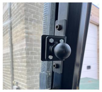
2. Place the square base over the mounting posts on the back of the console.
