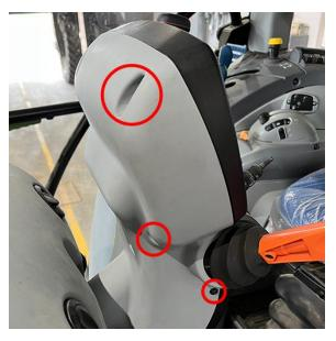
2. Remove the three screws located on the right side and back of the console.
