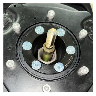
4. Rotate the motor so the electrical connector is at the 1 o'clock position.
