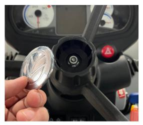
2. If the machine is equipped with a telescopic steering wheel, use a 13 mm socket to remove the hex nut.
