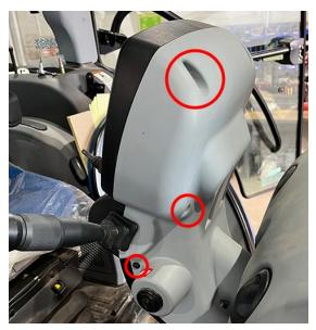
3. Remove the two screws located on the bottom of the front panel.
