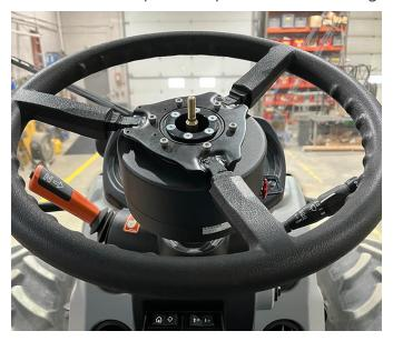
**Note:** If the splines do not easily connect, immediately stop and check spline alignment before proceeding.
