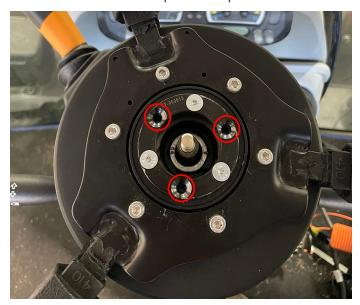
4. Attach an OTC 7403 steering wheel puller with M5  $\times$  0.8  $\times$  100+ mm bolts to the DirecSteer assembly. Use the provided spacer (P/N 305-1001-011) to protect the telescoping stem when applicable.
