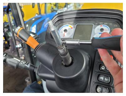
30. Ensure the steering column is fully extended to facilitate installing the DirecSteer assembly.
