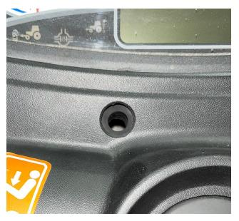
20. If the grommet is correctly aligned with the hole, remove the front cover and tighten the bolts securing the anti-rotation clamp.
