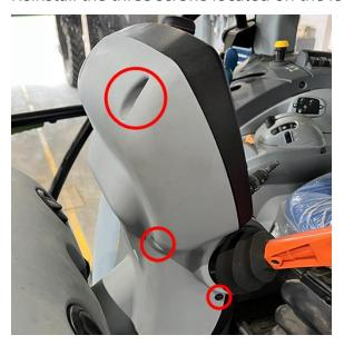
24. Reinstall the three screws located on the right side and back of the console.
