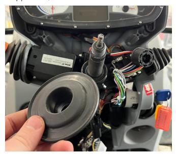
22. Reconnect the three connections between the front panel and the wire harness.
