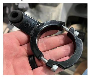
9. With the bevel side facing down, place the anti-rotation clamp around the steering column.
