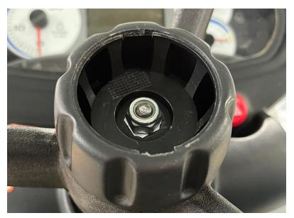
3. Remove the lock knob and spacer.
