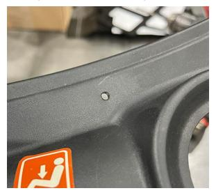
18. Increase the size of hole to 14.5 mm or 9/16 in wide with a step drill.
