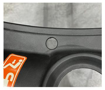
19. Replace the front panel and ensure the grommet is correctly aligned with the drilled hole.
