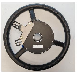
2. Carefully lower the DirecSteer assembly onto the steering shaft. Take care to ensure the teeth of the spline adapter and the steering shaft line up properly.
