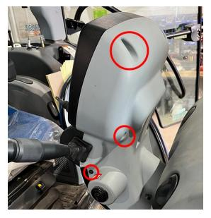
25. Reinstall the two screws located on the bottom of the front panel.
