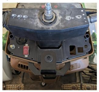
15. Reinstall the top cover and tighten the four bolts on the bottom of the dashboard.
