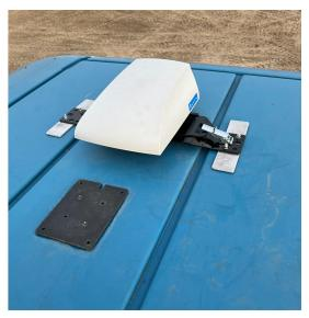
7. If applicable, mount the round adhesive plate for the LAIRD cellular antenna (P/N 121-0000-042) within 50 cm [20 in] from the antenna receiver bracket.
