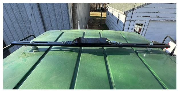
5. Attach and secure the antenna receiver onto the receiver bracket so that the antenna receiver is facing the front of the machine.
