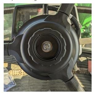
7. Install the cover of the knob on the steering wheel.
