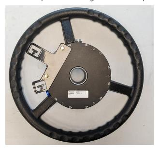
3. Attach the anti-rotation stem (P/N 063-4001-045) to the DirecSteer assembly at the 6 o'clock position with two of the provided bolts (P/N 311-4035-002K), but do not tighten.
