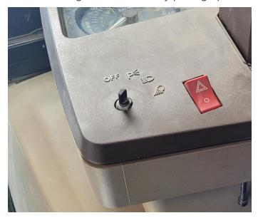
4. Remove the instrument cluster cover by lifting the bottom edge and then hinging it upwards.
