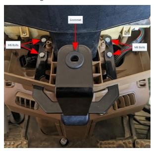
13. Reinstall the lower cover and connect the hazard switch, light switch, and the alarm speaker if applicable.
