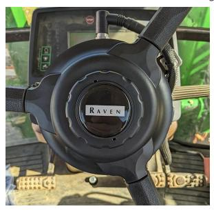
8. Check that all hardware is properly tightened and the DirecSteer is secure.
