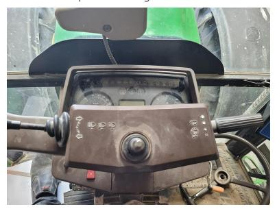
16. Reinstall the Light switch knob back on the dashboard to finish reassembling the dashboard of the tractor.
