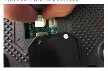
**Note:** The SIM card must be inserted into the J11 slot or the RS1<sup>m</sup> will not connect to wireless or a CORS network.
