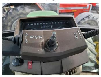
**Note:** The factory steering wheel and components will not be used with the DirecSteer system. It is recommended to keep these components in case the DirecSteer system will be uninstalled or moved to a different machine.
