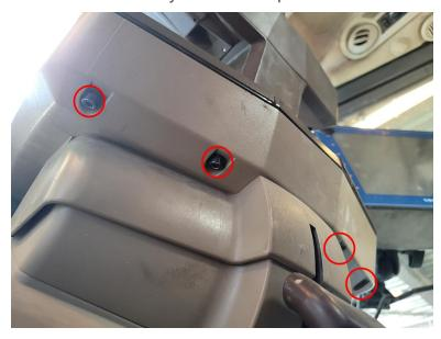
2. In 6x30/7x30 models, there is a glow plug indicator lamp on the dashboard, use a small flathead screwdriver to lift up and disconnect the lamp. See picture below for location.
