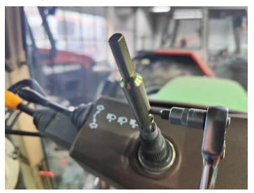
2. Install the DirecSteer assembly on the steering column while inserting the pin of the anti-rotation stem assembly through the grommet.
