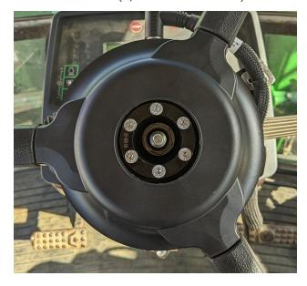
6. Install the included telescope locking knob (P/N 106-0159-783) on the telescope adapter and tighten the included M8 nut with a 13 mm socket.
