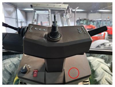
3. Remove the light switch knob by pulling up on it.
