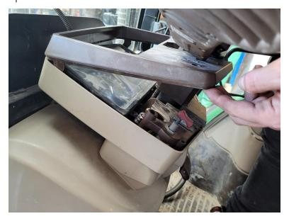
5. Use a #2 Phillips screwdriver to remove the two screws from the mid cover.
