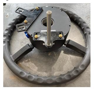
**Note:** The position of the anti-rotation stem may be further adjusted during installation. It is recommended to **not** tighten the bolts at this time.
