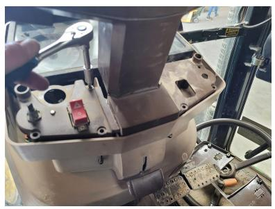
6. Unplug the hazard switch, light switch, and alarm speaker (if equipped).
