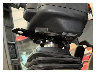
**Note:** The alignment of the column clamp may be further adjusted during installation. It is recommended to **not** tighten the hardware at this time.
