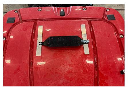
6. Attach and secure the antenna receiver onto the receiver bracket so that the antenna receiver is facing the front of the machine.
