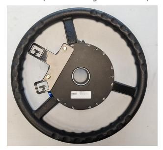
3. Attach the anti-rotation stem (P/N 063-4001-098) to the DirecSteer assembly at the 2 o'clock position with two of the provided bolts (P/N 311-4035-002K), but do not tighten.
