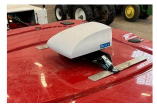
7. If applicable, mount the round adhesive plate for the LAIRD cellular antenna (P/N 121-0000-042) within 50 cm [20 in] from the antenna receiver bracket.
