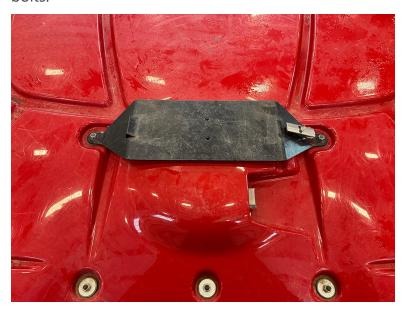
2. Attach the antenna receiver to the mounting bracket so that the front of the antenna is pointing to the front of the machine. Secure the antenna to the bracket with the latch.
