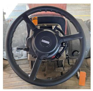
4. Tighten all anti-rotation hardware and brackets as needed.
