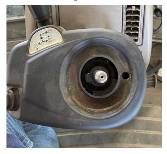
**Note:** The factory steering wheel and components will not be used with the DirecSteer system. It is recommended to keep these components in case the DirecSteer system will be uninstalled or moved to a different machine.
