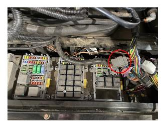
12. Connect motor cable (P/N 115-4001-258) to the electrical port on the DirecSteer assembly.
