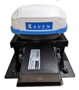
7. Attach the roof bracket (P/N 116-4001-001) to the RS1 $^{\rm m}$  fixed mount bracket (P/N 107-0172-498) with the provided four M6 x 16 countersink screws (P/N 311-4073-134) using a 4 mm hex key.
