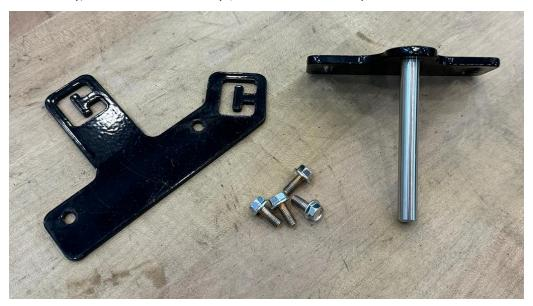
2. Attach the cable routing bracket (P/N 107-4001-093) to the DirecSteer assembly at the 10 o'clock position and tighten with two provided M5 x 12 bolts (P/N 311-4035-002K).
