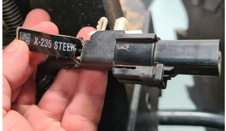
Figura 10 - Conector "X-235 STEERING ANGLE SENSOR"
