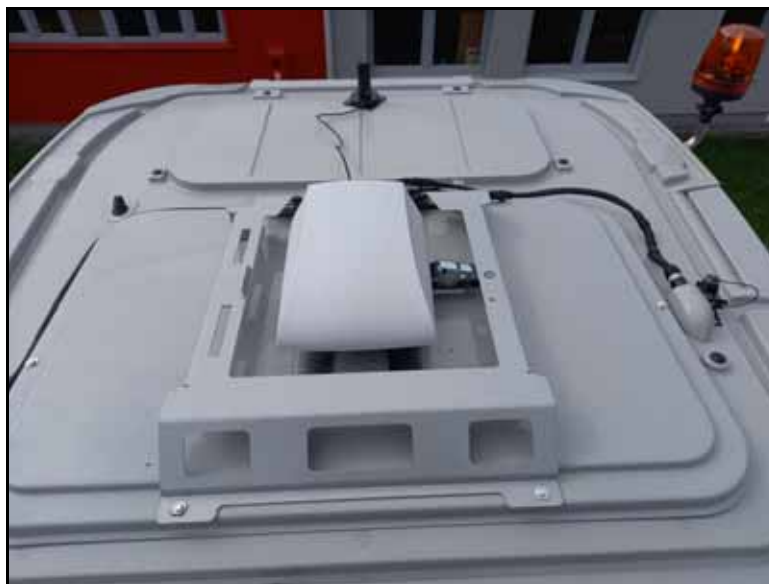
FIGURE 7. RS1™ Mounted and Cable Connected
