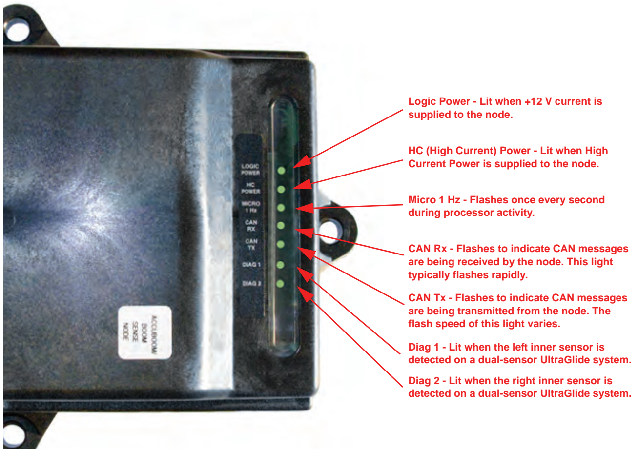
FIGURE 1. AccuBoom CAN Control Node LEDs
