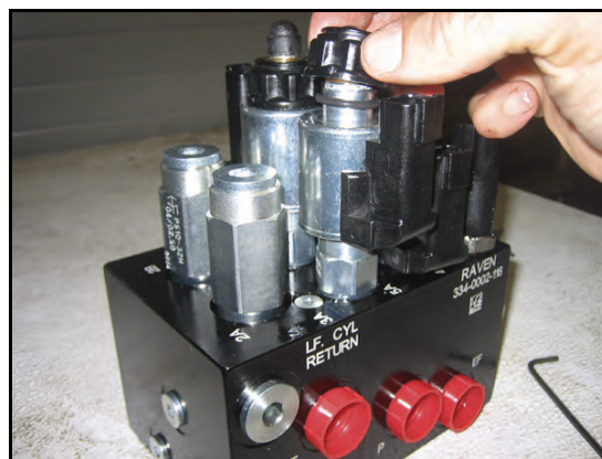
FIGURE 20. Coil Reinstalled on the AutoBoom Valve
