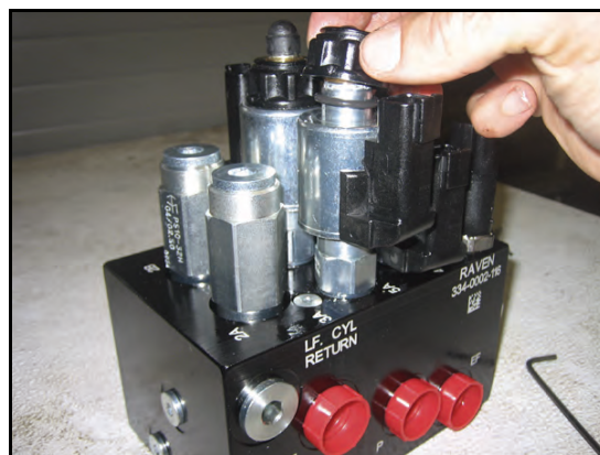
FIGURE 19. Coil Reinstalled on the AutoBoom Valve
