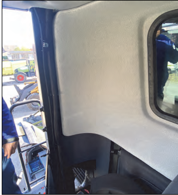
FIGURE 8. B-Pillar and Corner Trim Panels Removed
