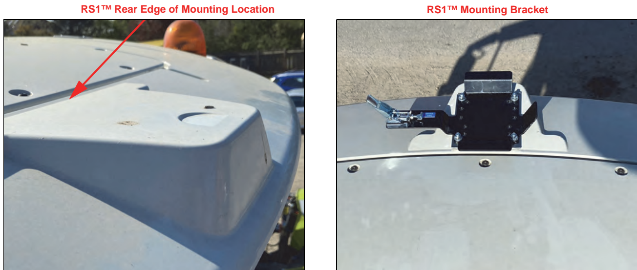
FIGURE 9. RS1™ Roof Top Mounting Location
