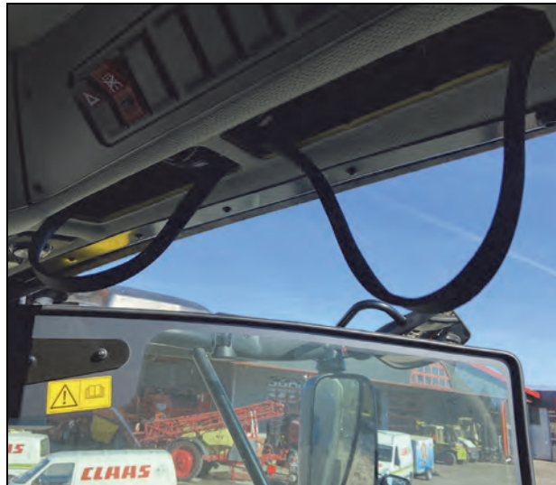
FIGURE 13. Route the RS1 Cable Through the Cab Ceiling
