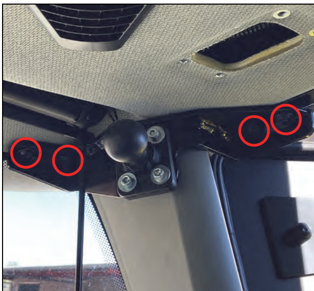
FIGURE 12. Display Bracket Mounted
