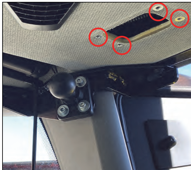
FIGURE 14. Display Connector Ceiling Plate Mounting Location
