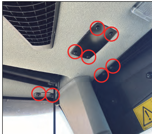
FIGURE 10. A-Pillar and Plate Screws
