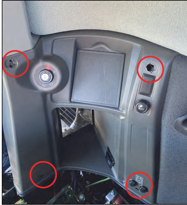
FIGURE 4. Lower Corner Panel Cap and Screw Locations
