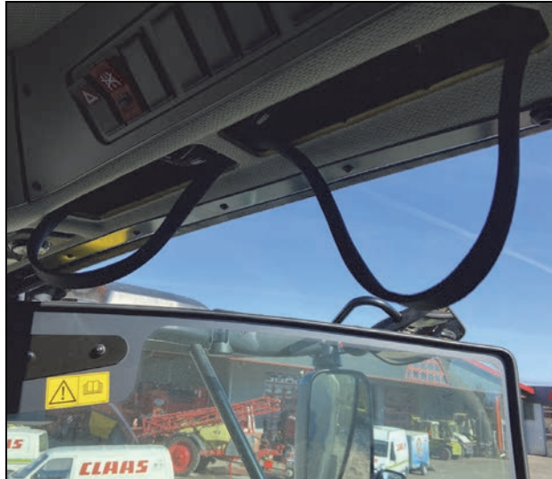
FIGURE 20. Route the Field Computer Cable
