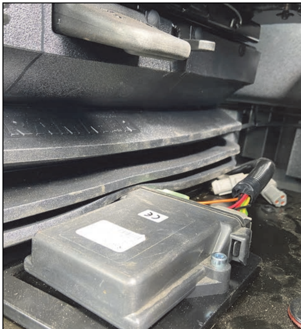
FIGURE 19. Smart Antenna Cable Connection
