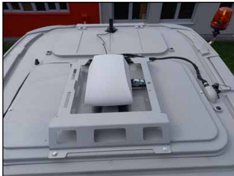
FIGURE 8. RS1™ Mounted and Cable Connected
