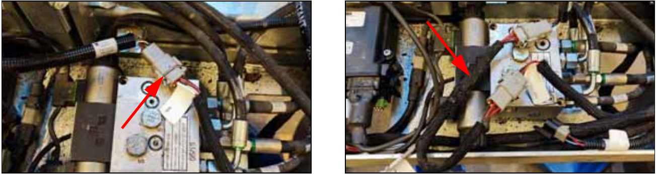
FIGURE 4. RTK Corrections T-Cable (P/N 115-4020-002) connected to Implement SC1 cable and Smart Antenna Cable
