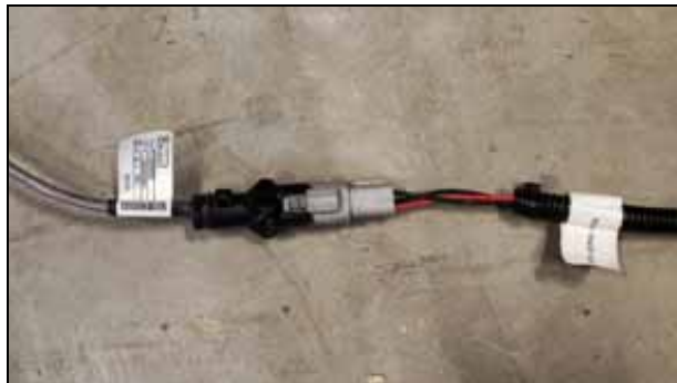
FIGURE 5. 3-pin to Serial cable (P/N 115-0172-448) connected to RTK Corrections cable
