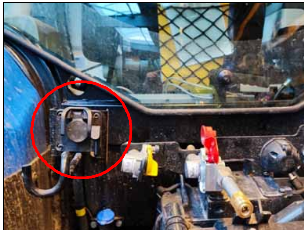
FIGURE 3. Implement Bus Breakaway Connector on the back of the tractor
