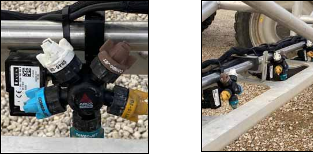
FIGURE 2. Hypro Left-Handed Nozzle Bodies Installed
