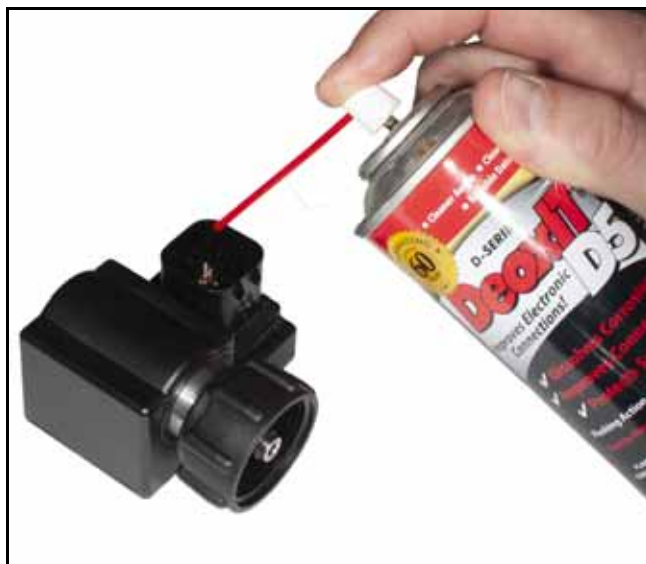
FIGURE 1. DeoxIT D5 Applied to Hawkeye® 2 NCV
