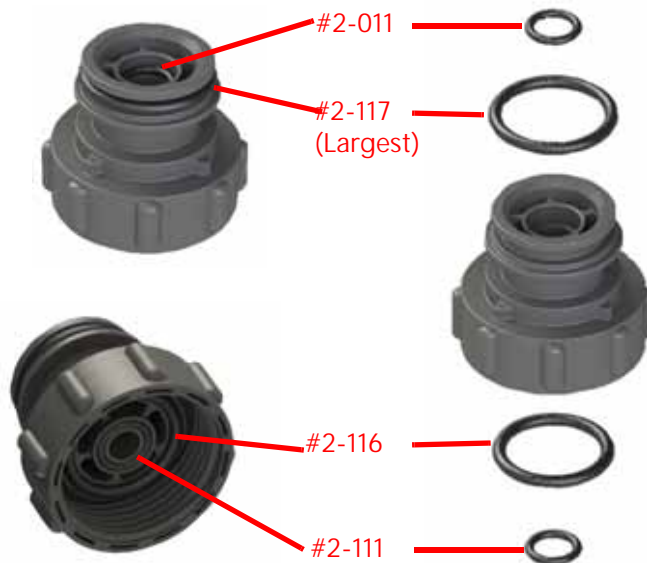
FIGURE 3. ProStop-E Adapter O-Ring Installation
