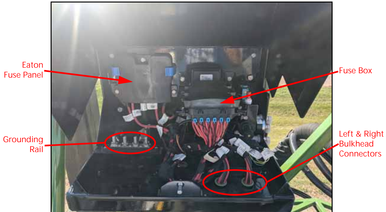
FIGURE 2. Power Distribution Cabinet with Hawkeye® 2 Installed
