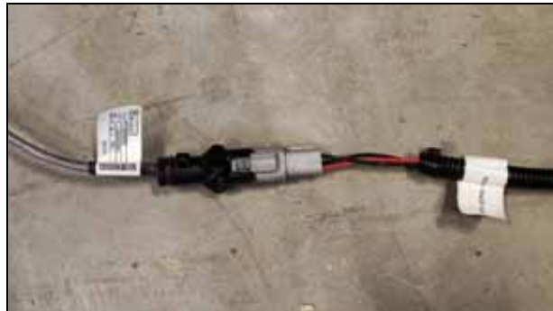
FIGURE 3. 3-pin to Serial cable (P/N 115-0172-448) connected to RTK Corrections cable
