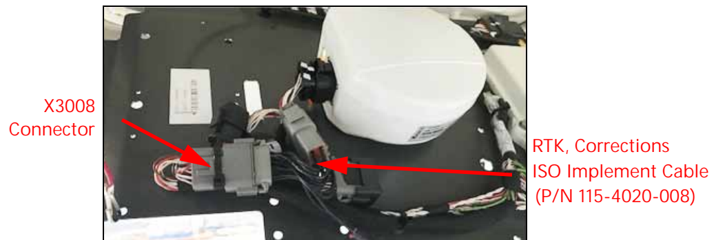
FIGURE 5. RTK Corrections ISO Implement cable (P/N 115-4020-008) connections.
