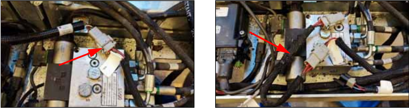
FIGURE 2. RTK Corrections T-Cable (P/N 115-4020-002) connected to Implement SC1 cable and Smart Antenna Cable
