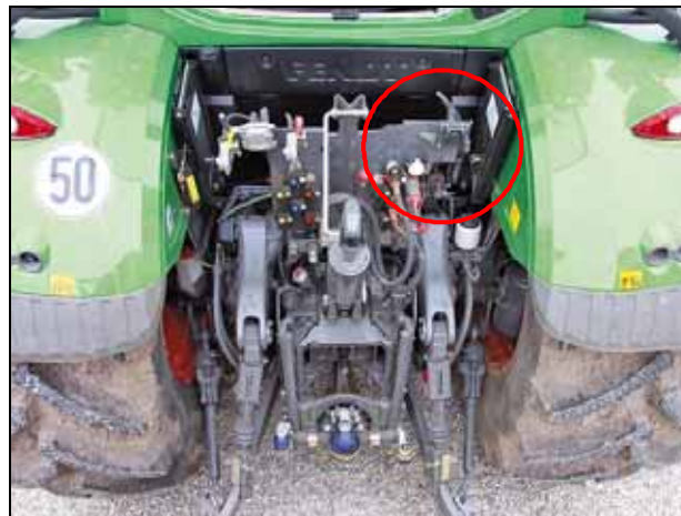
FIGURE 1. Implement Bus Breakaway Connector on the back of the tractor
