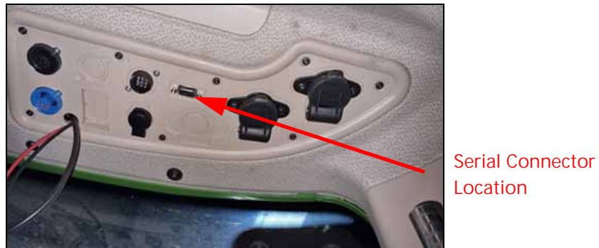
FIGURE 6. Overhead Connector Panel on Right Side of Cabin
