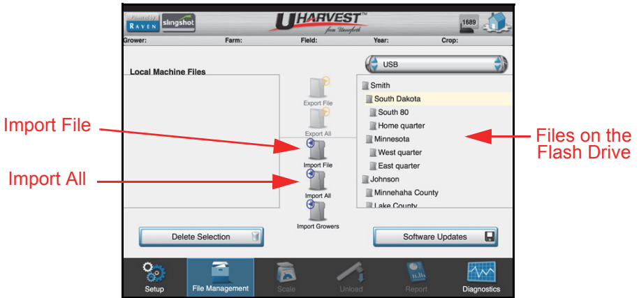
FIGURE 44. Import Files to the Processor
