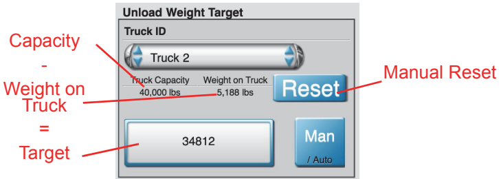
FIGURE 20. Target Weight Calculation
