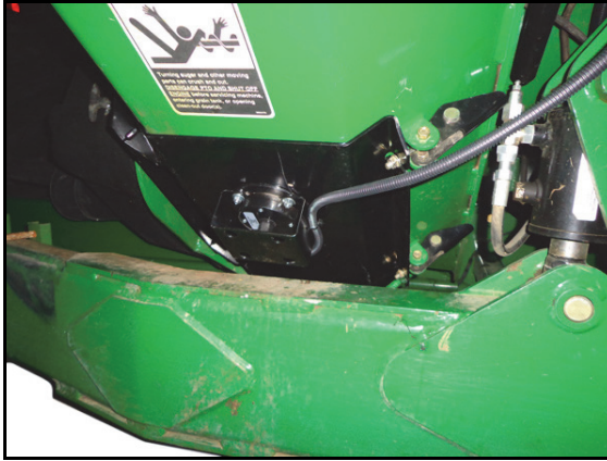
FIGURE 8. Moisture Sensor on Cleanout Door
