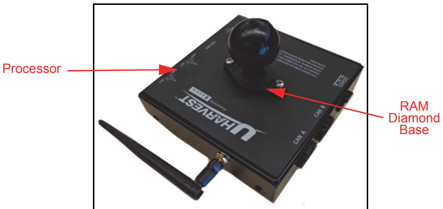
FIGURE 1. RAM Diamond Base attached to Processor
