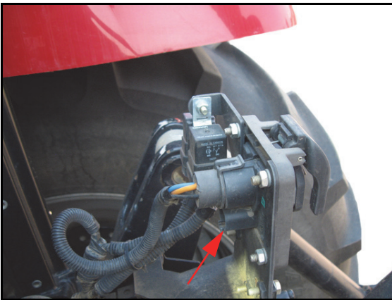
FIGURE 5. Deutsch 4-Pin Connector Removed
