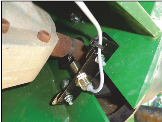
FIGURE 6. PTO Sensor and Target
