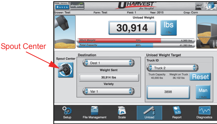
FIGURE 34. Spout Center Icon on Unload Screen
