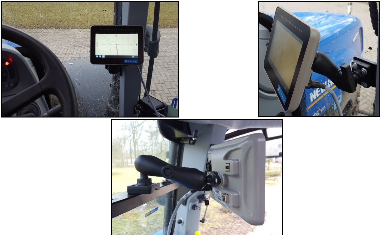
FIGURE 6. Example of CR12™/V4 Mounted in Various Positions
