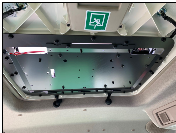
FIGURE 2. Roof Hatch Lining Removed
