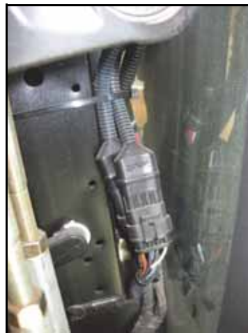
FIGURE 5. Removed Shroud from Steering Column
