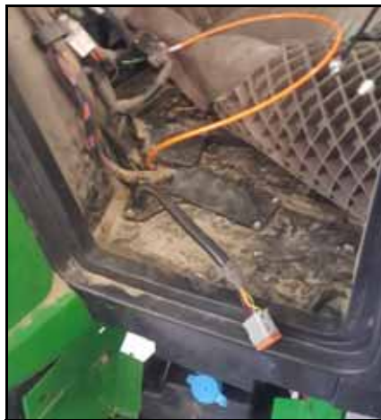
FIGURE 12. Cable Routed through Cab Floor
