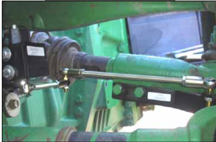
FIGURE 11. Installing Raven WAS
