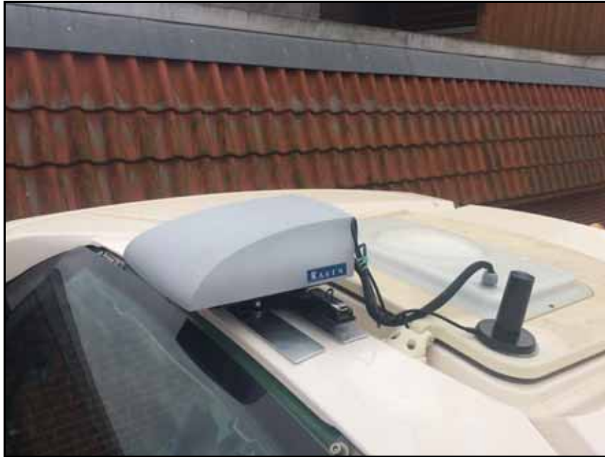
FIGURE 17. Laird Antenna Adhesive Plate
