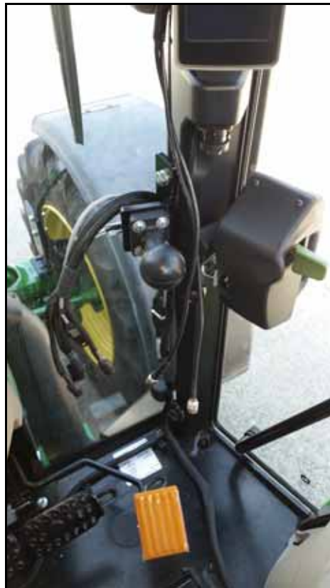
FIGURE 21. Field Computer Harness from Floor to A-Pillar
