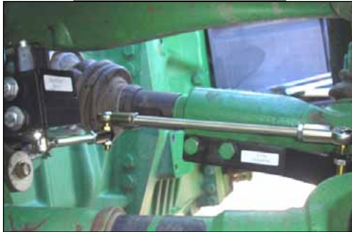
FIGURE 11. Installing Raven WAS
