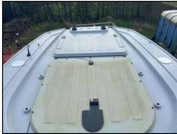
FIGURE 21. GPS Patch Antenna and Two GPRS/UMTS Antennas
