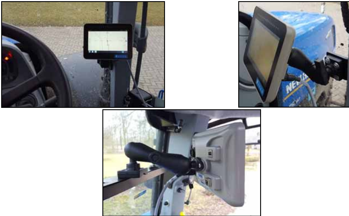
FIGURE 24. CR12 Mounting Examples
