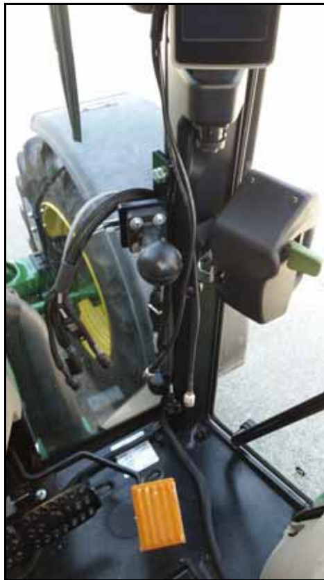
FIGURE 14. Field Computer Harness from Floor to A-Pillar
