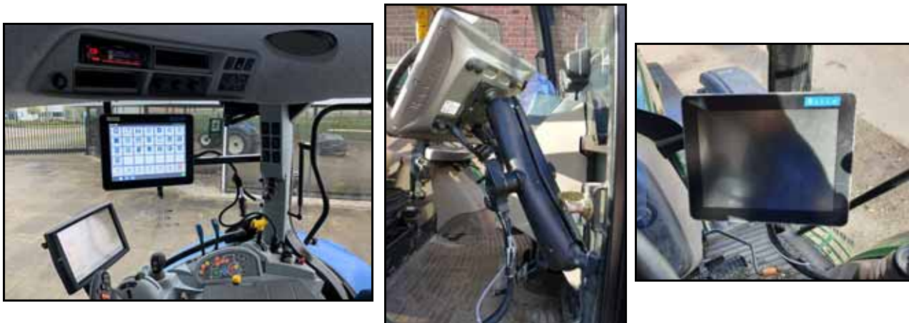
FIGURE 24. CR12 Mounting Examples
