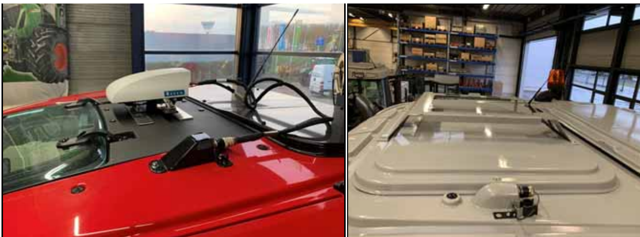
FIGURE 4. RS1 Mounted and Cable Connected
