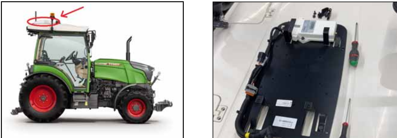
FIGURE 2. Roof Cover and Roof Plate Removed
