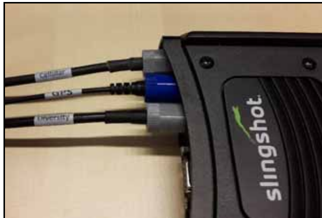
FIGURE 9. Labeled Antenna Cables with SMA Grips
