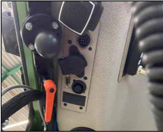
FIGURE 16. ISOBUS and Power Connector
