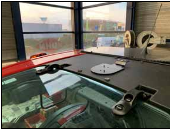
FIGURE 8. 700S Mounting Plate and Antenna
