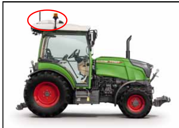
FIGURE 5. Roof Cover / AGCO Guidance Controller Plate
