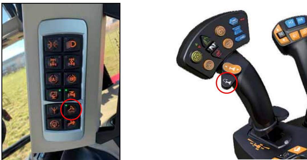
FIGURE 12. Pre-Activation Button on C-Pillar
