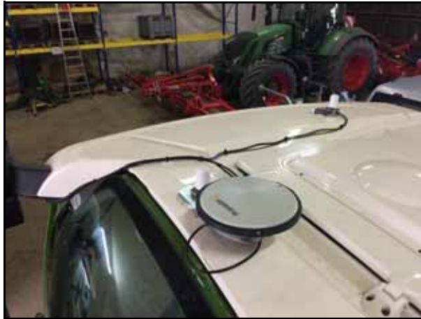
FIGURE 11. GPS Patch Antenna and Two GPRS/UMTS Antennas
