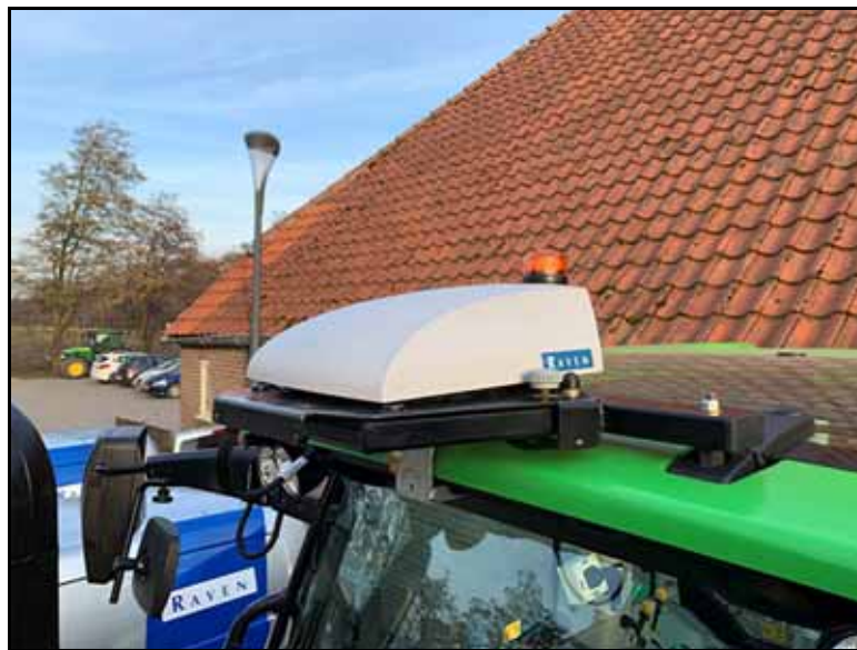
FIGURE 5. RS1™ Mounted and Cable Connected
