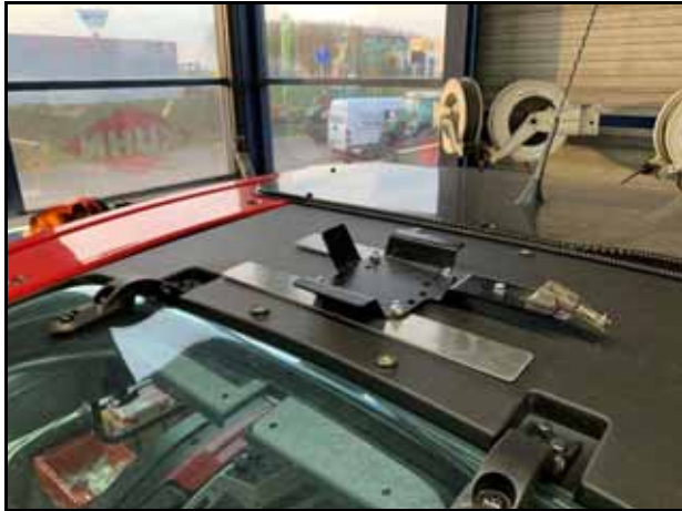
FIGURE 2. Bottom Assembly of RS1™ Mount
