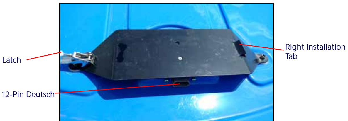
FIGURE 2. Right Installation Tab
