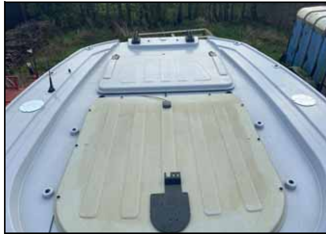
FIGURE 10. GPS Patch Antenna and Two GPRS/UMTS Antennas
