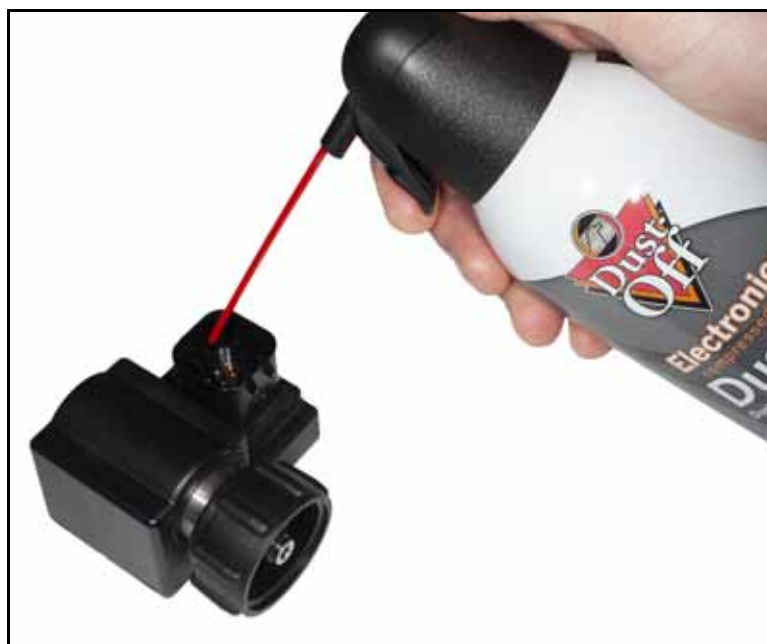
FIGURE 3. Compressed Air Used to Dry Connector
