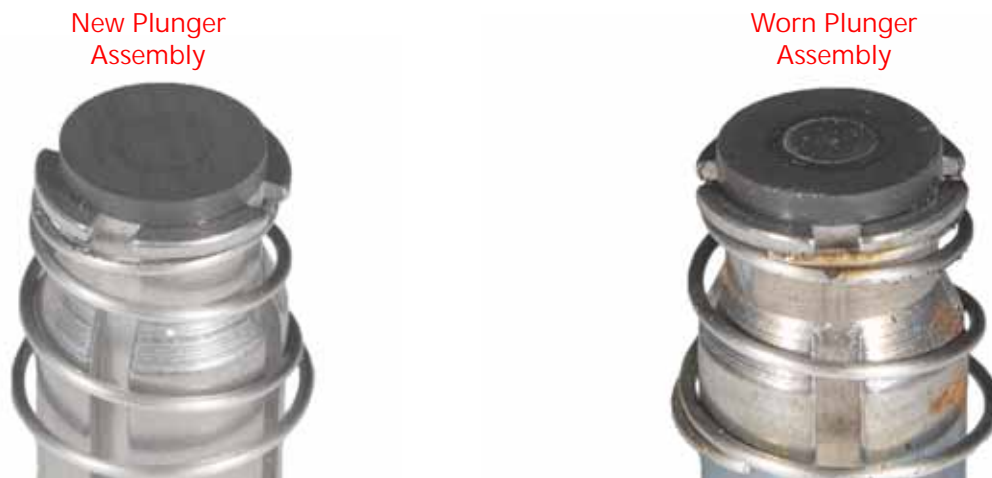
FIGURE 4. Plunger Inspection Detail
