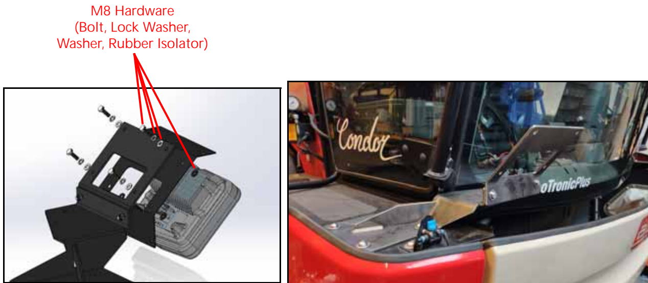
FIGURE 3. VSN Camera and Mounting Bracket Assembly
