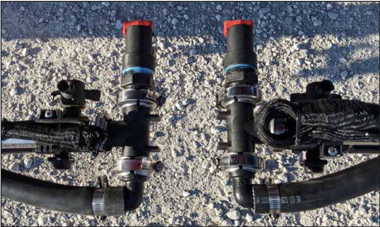
FIGURE 10. Center Boom Section Plumbing Routing Example
