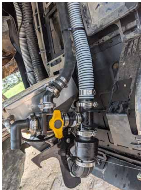
FIGURE 7. Drain Valve and Drain Hose for Remote Educator Mounting Option
