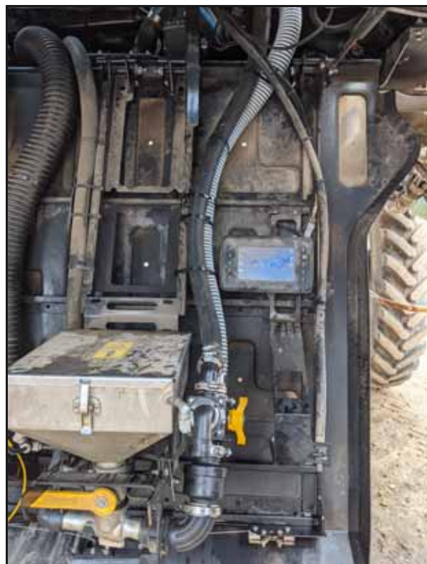
FIGURE 7. Drain Valve and Drain Hose for Remote Educator Mounting Option
