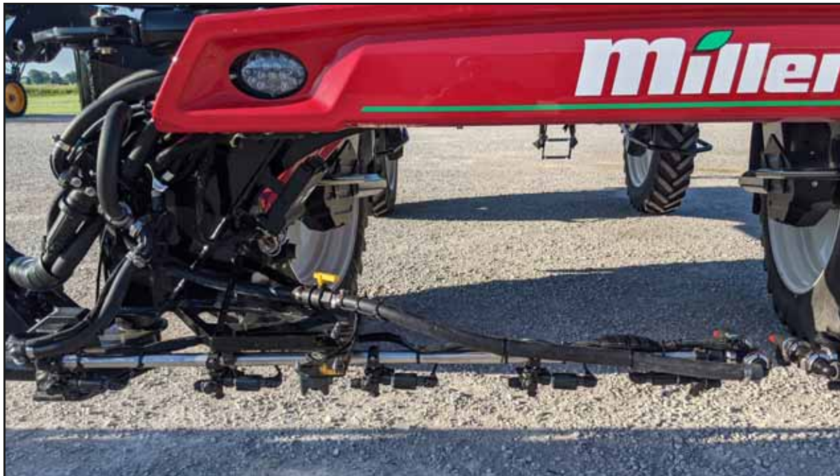
FIGURE 10. Center Boom Section Plumbing Routing Example
