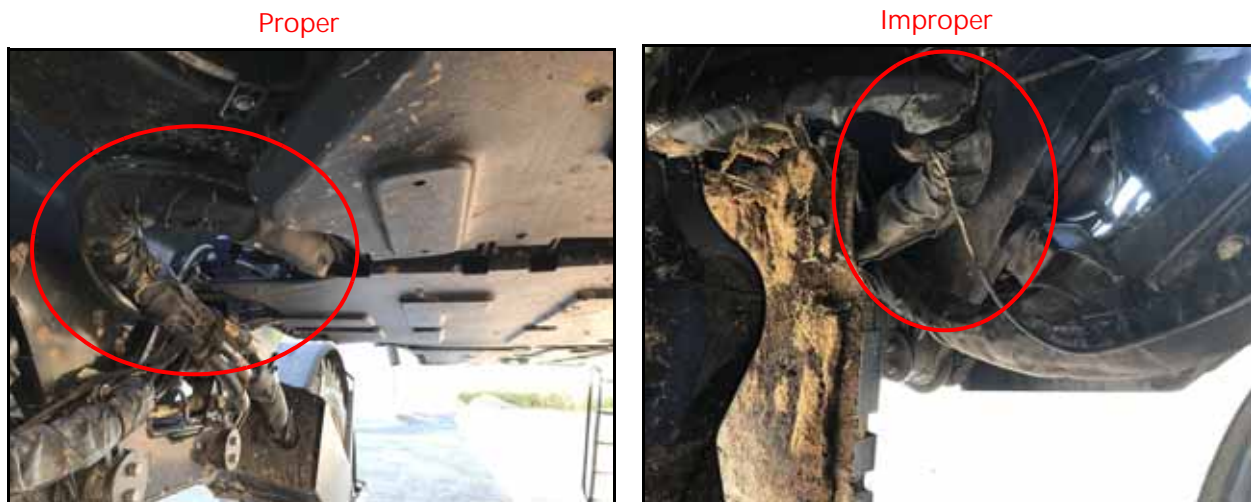
FIGURE 4. Proper and Improper Cable Routing
