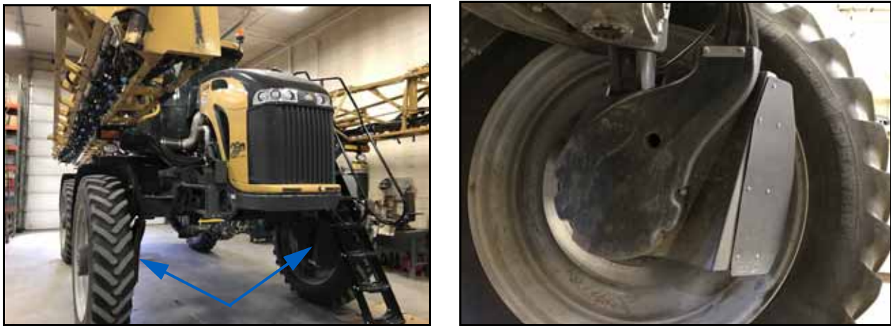
FIGURE 2. Removed Wheel Motor Cover
